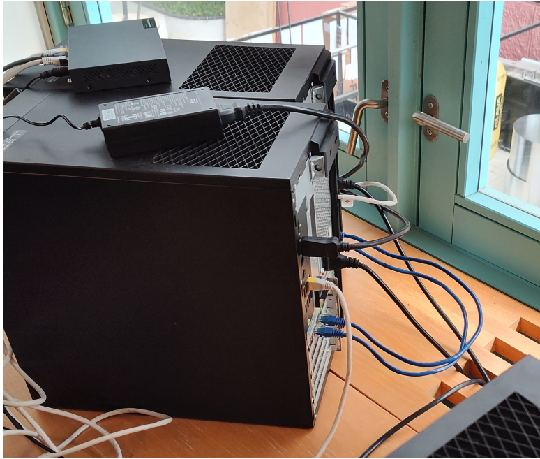
Figure 3.1: Photo of testbed setup, with the PGEN and DUT connected directly to each other
