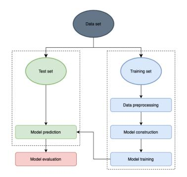
Figure 2.4.2: Flow chart machine learning model construction. Inspired by: [31]
