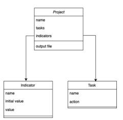
Figure 3.2.1: The main classes of the simulator.
