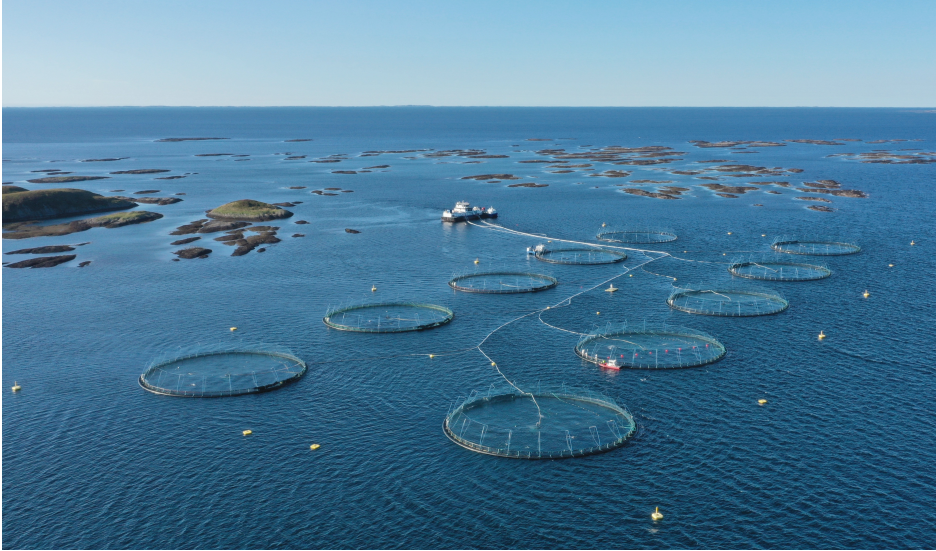
Figure 1.1: Example of a salmon production site with 10 cages (Tristeinen, Tarva municipality, Norway). The frame mooring system is outlined by the yellow buoys, and the feed barge is seen in the background. Image credit: SINTEF ACE (SINTEF ACE, 2023).
