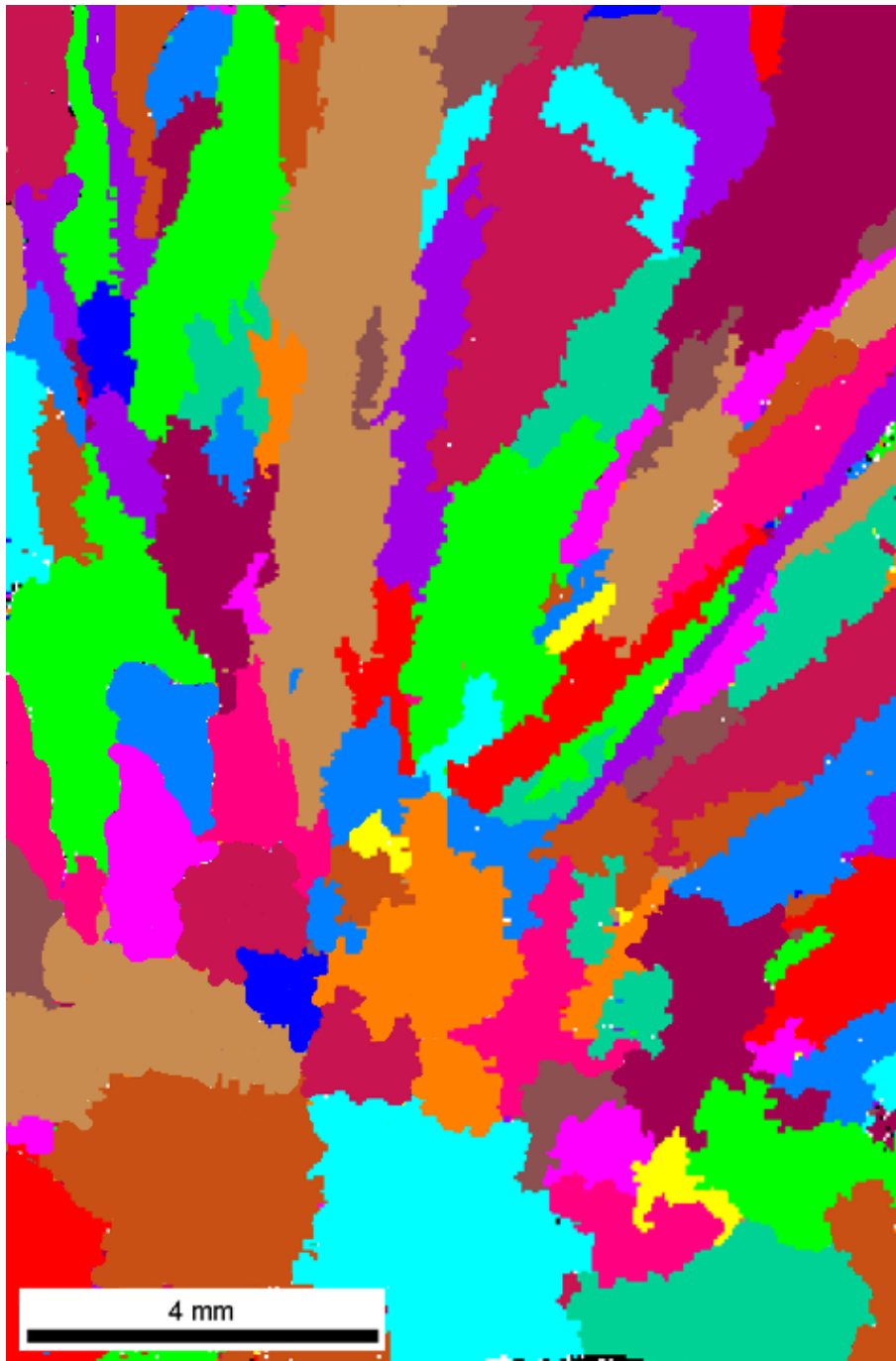
Figure 28: EBSD map of thermal analysis cup sample without EGR.
