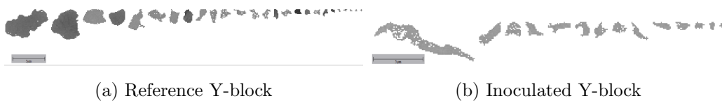
Figure 45: Uncharacterized/other inclusions in the reference and inoculated Y-block samples.
