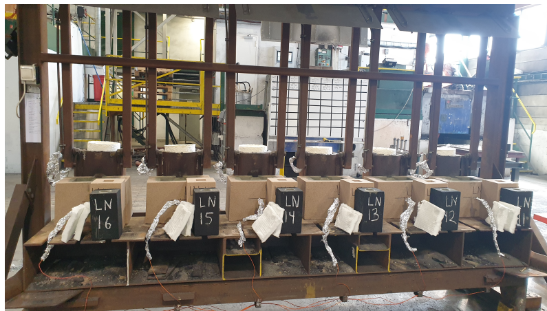
Figure 16: Rig setup. Casting order from right to left.
