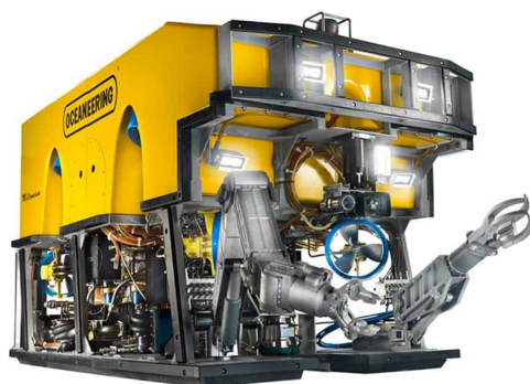
Figure 3.3.: The Millennium® Plus ROV from Oceanering - it has manipulators and grippers/end-effectors that can grab structures, move components, turn valves and more.[18]
