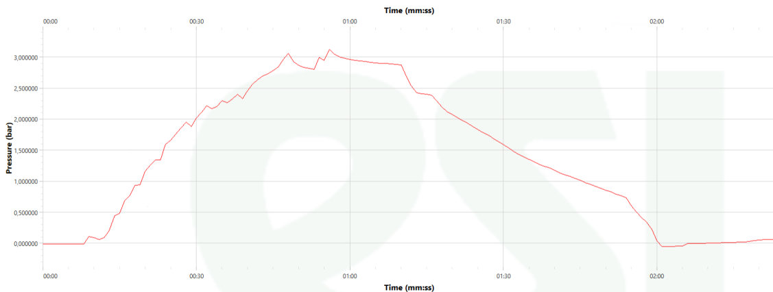
Figure 4.16: Change in pressure inside the rubber bellow, Shore 70, during test 7.5
