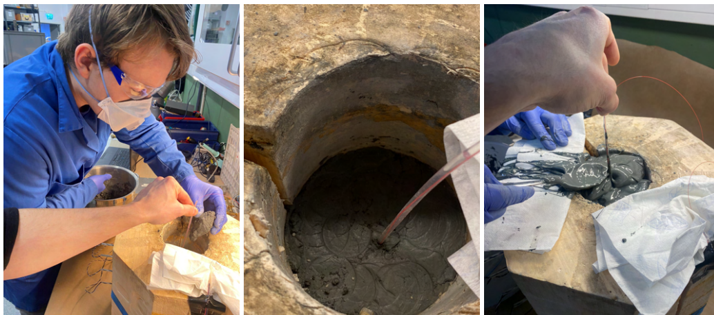
(a) Lumps of stabilized clay (b) Tamped stabilized clay (c) Remoulded quick clay
