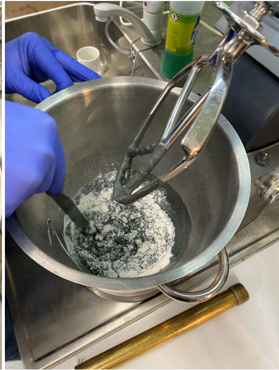
(b) Mixing of quick clay and lime
