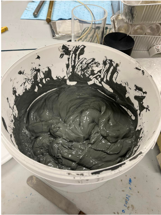
(a) Bucket of quick clay remoulded by hand
