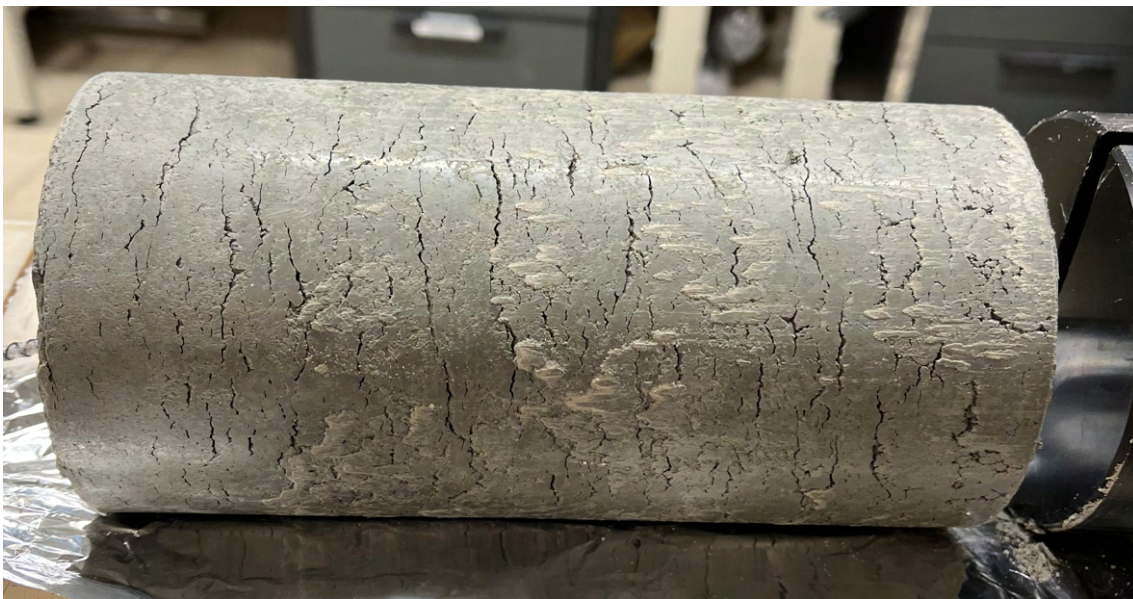
Figure 10.5: Sample 2 straight after it had been pushed out of the plastic cylinder it was cured inside. A lot of small cracks and imperfections can be seen.
