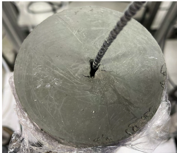
Figure 10.3: A crater at the top of Sample 2 causing no bonding in this upper area. The same situation was observed at the bottom.
