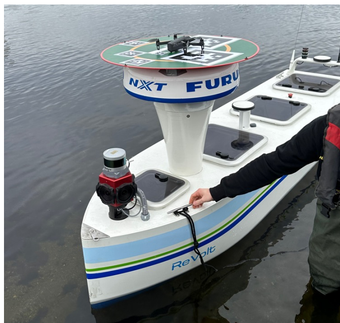
Figure 3.6: Helipad mounted on ReVolt. Image courtesy of Tom Arne Pedersen from DNV
