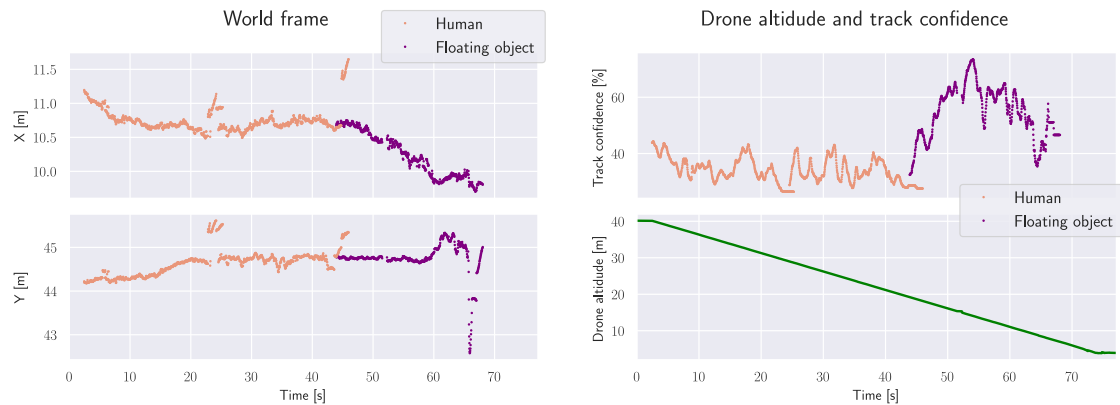
Figure 5.16: Search YOLO network detections under slow descent from 40m to 3m with a human in the water
