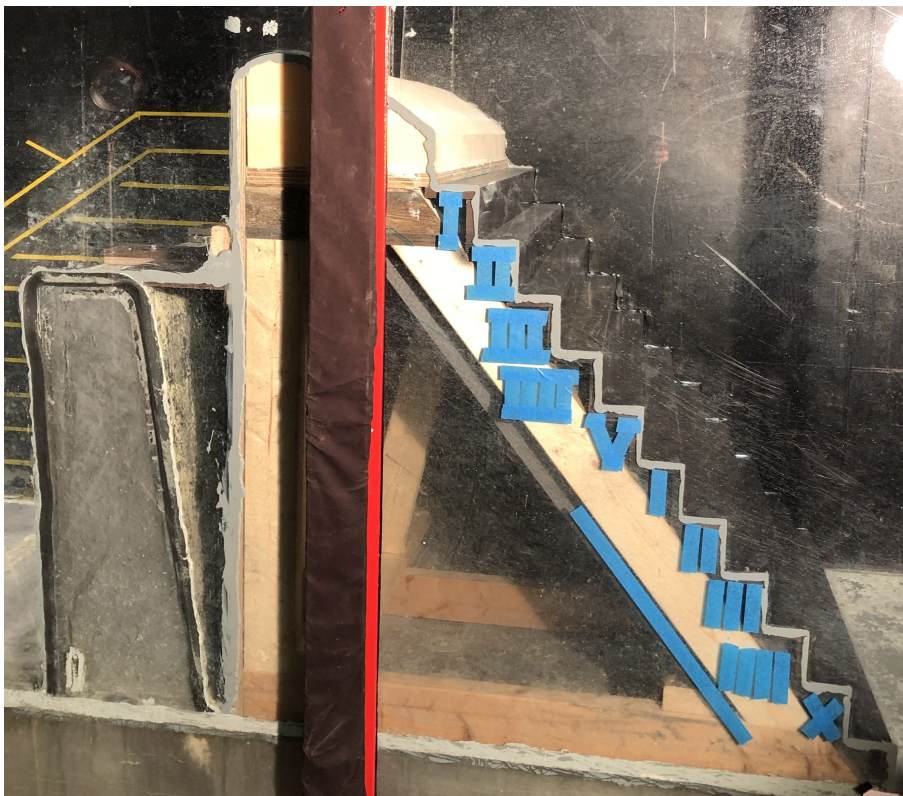
Figure 3.1.3: D-model scaled 1:16.67 with a total height of 1.20 meters seen from the side through the glass wall of the D-flume.
