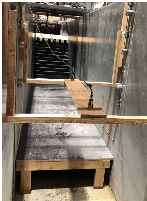
Figure 3.2.3: Looking upstream in the D-flume, ultrasonic sensors for measuring the sequent depth of the hydraulic jump are seen in the front. The wood construction on the bed downstream of the toe is to ensure an undisturbed development of the hydraulic jump. The D-model with splitters can be seen in the background.
