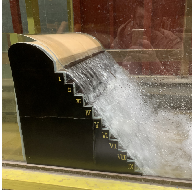
Figure 4.1.2: A nappe from the first step is formed for very low discharges, here shown in the C-model basecase - h_c/h_s = 0.6 .
