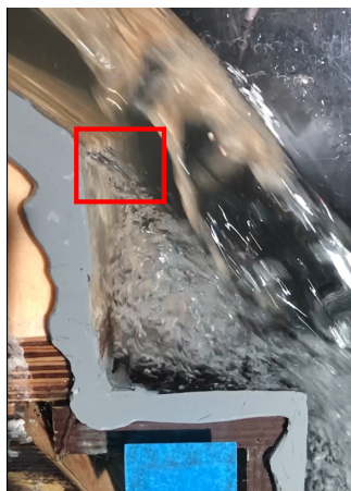
Figure 4.5.1: Region of low pressure on spillway surface in D-model.
