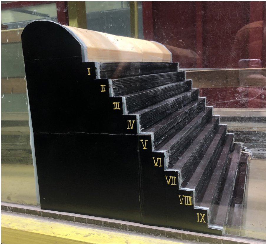
Figure 3.1.4: C-model scaled 1:50 with a total height of 0.40 meters seen from the side through the glass wall of the C-flume.
