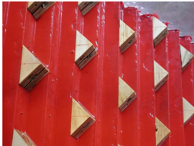
Figure 2.3.1: Physical model of stepped spillways with triangular protrusions (Wright 2006), flow direction from left to right.
