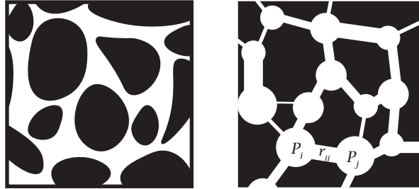
Figure 2.1: Illustration of the core idea of a pore network model. The left image represents a realistic 2D porous media with the solid material colored in black and the pore space in white. The right image represents a pore network model of our small sample, capturing the average flow properties of the real sample.
