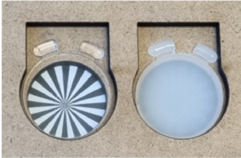
Figure 3.1: Test samples. \text{SiO}_2 concentration of 0.002% (left) and \text{SiO}_2 concentration of 0.3% (right)
