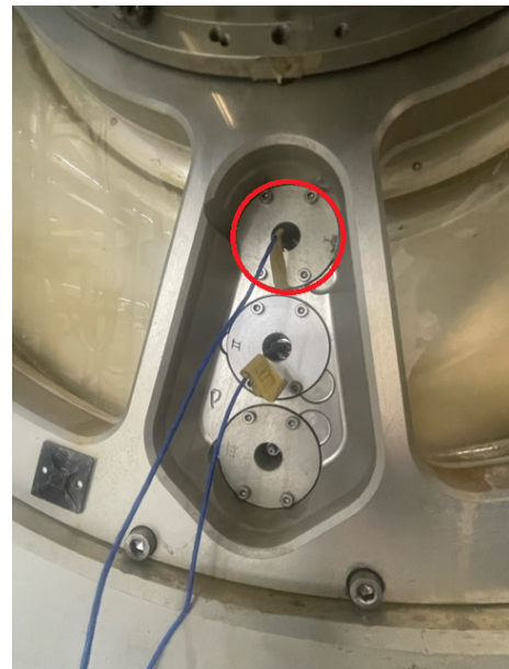
(b) Dynamic pressure sensor at the impeller outlet.
