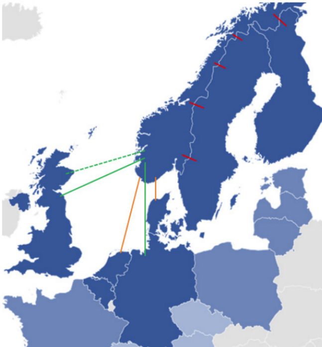
Figure 3.5: The electrical connections between Norway and other countries. AC (red), existing HVDC (orange), HVDC under construction (green), HVDC currently under consideration (green stippled). [59]
