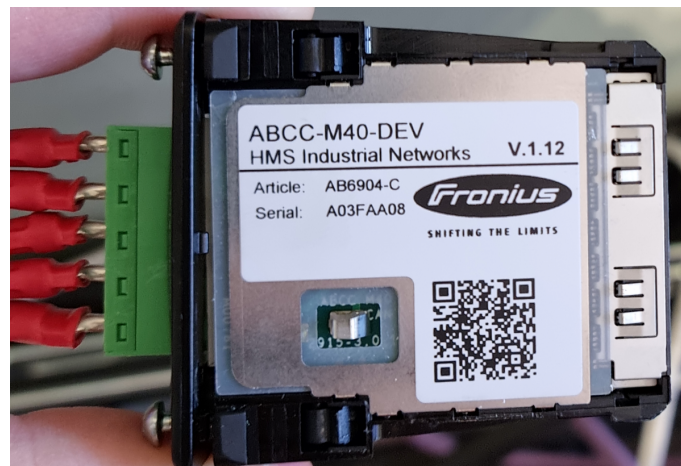
Figure 40: The DeviceNet Bus Card, which is used with the Robot Interface with the Fronius Welding Machine.
