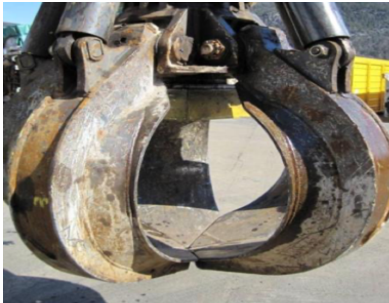
Figure 8: Excavator with Triple Claw (Internal Source with Permission from AF Offshore Decom)
