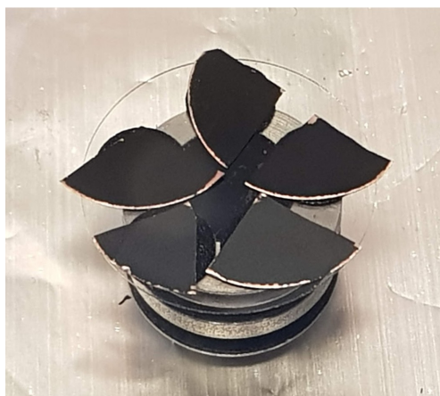
Figure 3.5: Image of the cut electrodes placed on the sample holder before being inserted in the XPS transfer arm.
