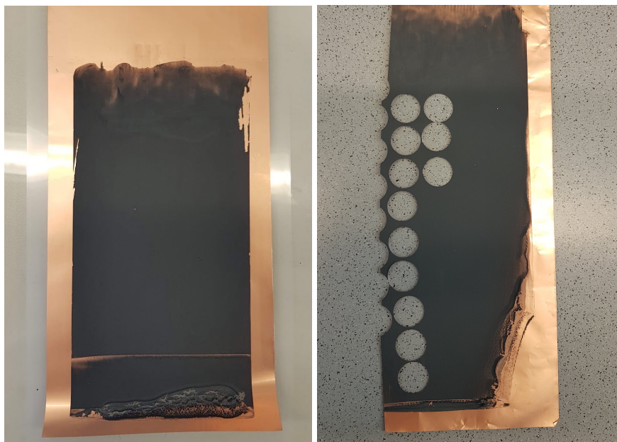
(a) Electrode cast on copper foil after drying. (b) Electrode cast after punching out electrodes.
