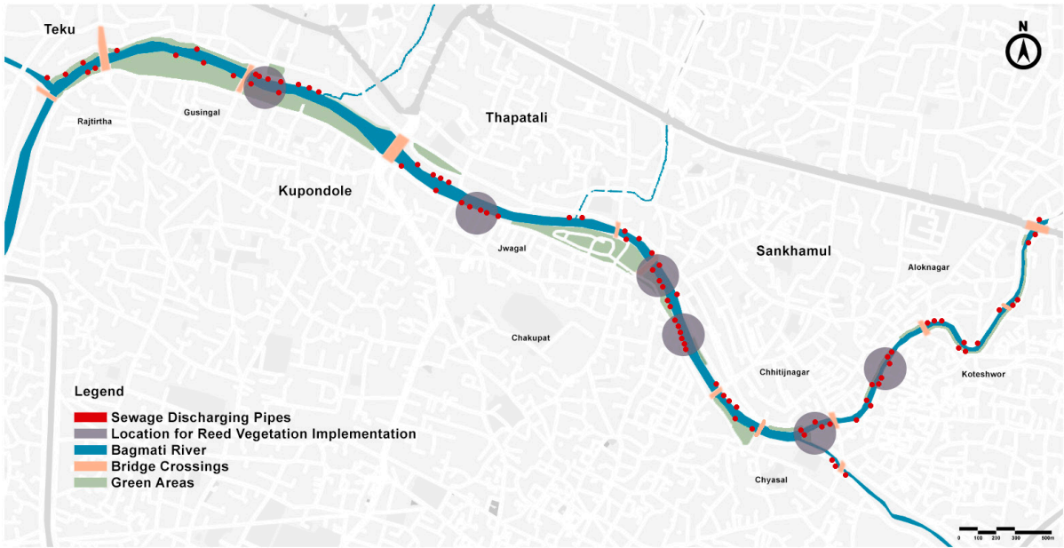
Fig 71. Optimal locations for implementation of Ecological Solution Reed Vegetation (Source: Self-made by author, 2023)
