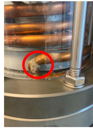
Figure 5-5: Flux used in the soldering
