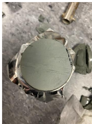
Figure 5-17: GDS sample ring with clay
