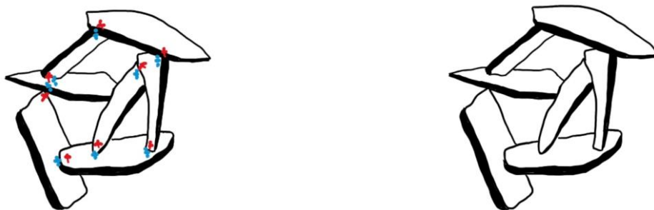
(a) Marine clay with saline porewater: stable structure, large attractive forces between particles edges and planes. There are small repulsive forces between particle planes
