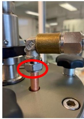
Figure 5-4: Connection between the hose and the copper coil
