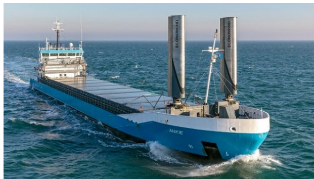
Figure 2.8: Suction wing installed on general cargo vessel Ankie (Chou et al., 2020)
