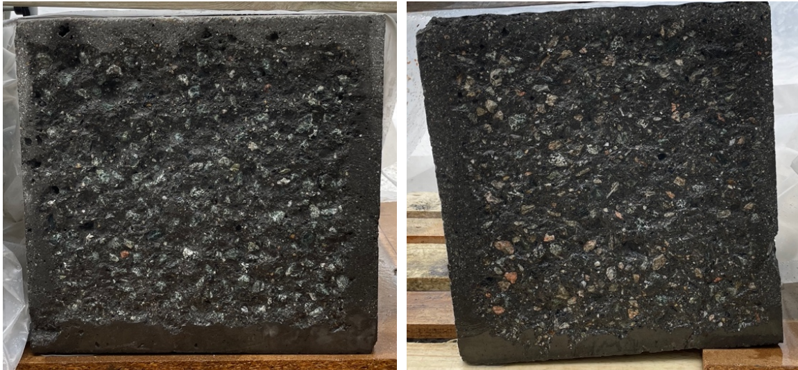
Figure 5-5: Main concrete castings for bond strength tests: Side A (GBS left, FWT right) after high pressure washing
