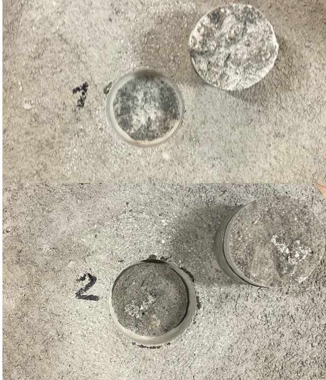
Attachment 6: Picture documentation and description of failure pattern from bond strength tests on dry shotcrete repair of GBS concrete
