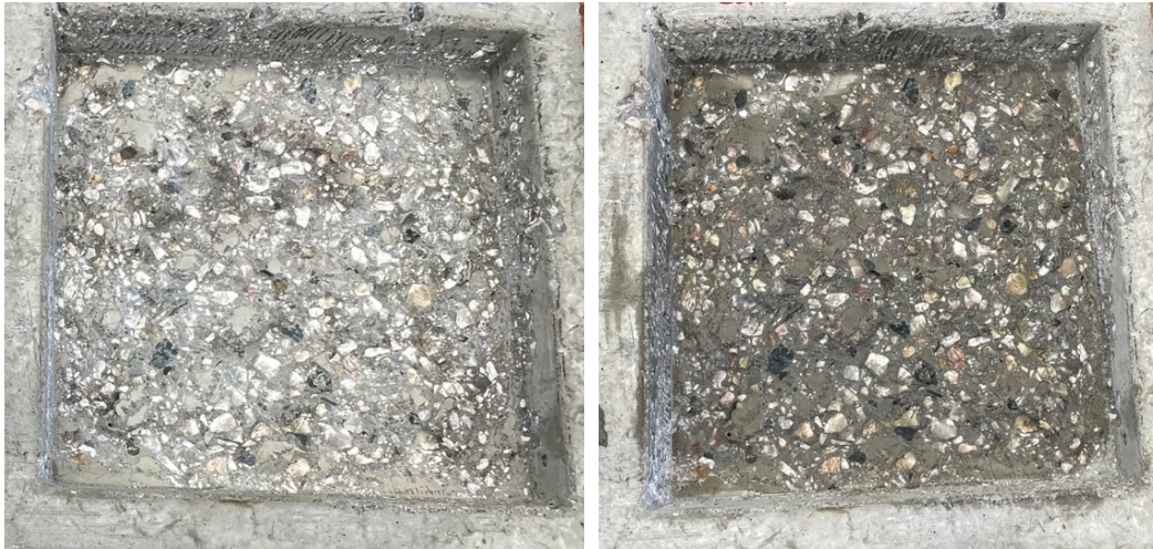
Figure 4-5: Concrete at a dry state (left) and at a saturated surface dry state (right)
