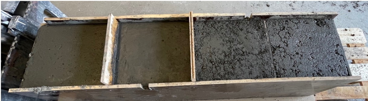
Figure 5-2: Main concrete castings for bond strength tests, GBS (left) and FWT (right)
