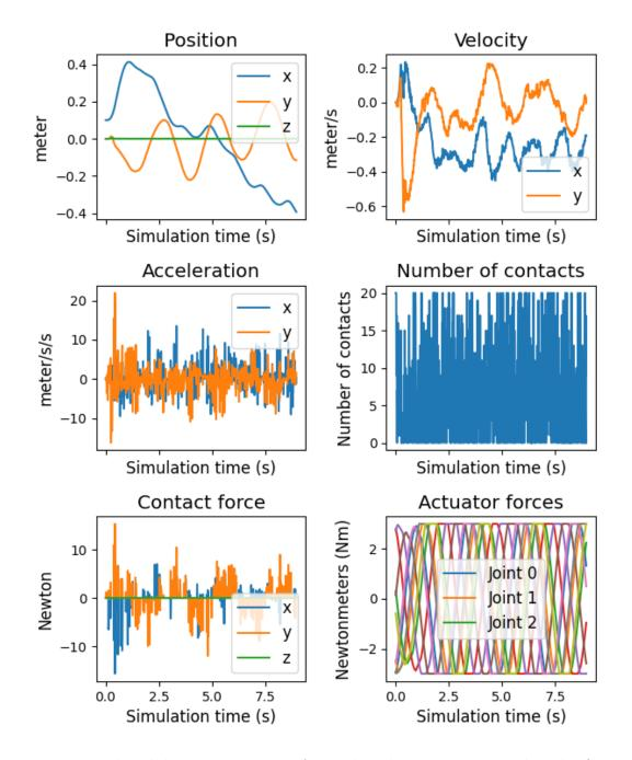
Figure 31: Lateral undulation experiment for snake robot over 10 seconds. The first row of the plot shows the head's position and velocity during the experiment. The second row shows the head's acceleration and the total number of contacts present in the simulator at any given time. The third row shows the measured contact forces for the head during the experiment as well as the actuator forces for each actuator.
