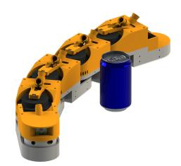
Figure 4: The Boa snake robot, courtesy of [5]
