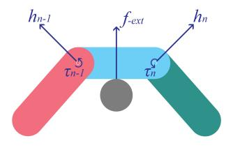
Figure 1: Forces and torques applied on a 2-jointed 2D-snake pushing up against an object. Courtesy of [5].
