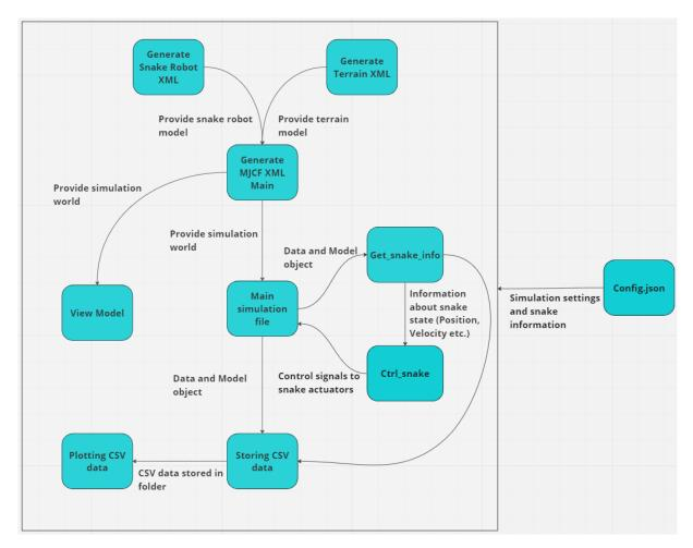
Figure 14: Software diagram explaining relationships between the different modules in the program. The four main modules are the simulation module, the configuration module, the XML generation module, and the data acquisition module
