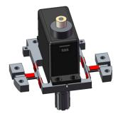
(a) 3D-model of an older version(v0) of the force-torque measurement system
