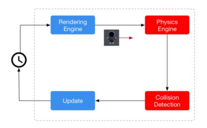
Figure 7: The simulation loop where the rendering engine is marked blue and the physics engine is marked red. Courtesy of [10]
