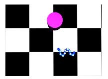
(a) Snake placement during the beginning of lateral undulation experiment. The white dots on the snake are the actuators changing color based on how much torque is being used from  $0 - \pm 3Nm$
