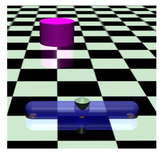
Figure 22: Configuration one showcasing a 2-linked snake. The object in the middle of the snake is an actuator that has been set to be visible to showcase the joint
