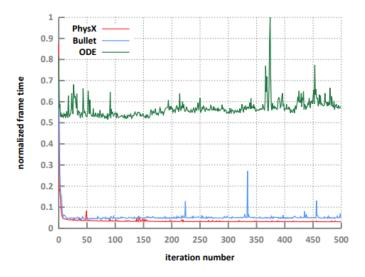
Figure 13: Frame rate comparison of PhysX, Bullet and ODE when dropping 625 spheres. Test conducted in 2012 which should be taken into consideration. Courtesy of [19]
