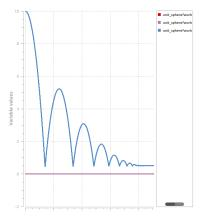
(a) Position graph for bouncing ball with ODE created using Gazebos built in graphing tool
