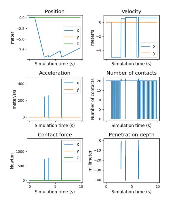
Figure 28: Collision test for ten linkages with a collision along the x-axis. The first row of the plot shows the head's position and velocity during the experiment. The second row shows the head's acceleration and the total number of contacts present in the simulator at any given time. The third row shows the measured contact forces for the head during the experiment and how far the head penetrated the cylinder during the collision.
