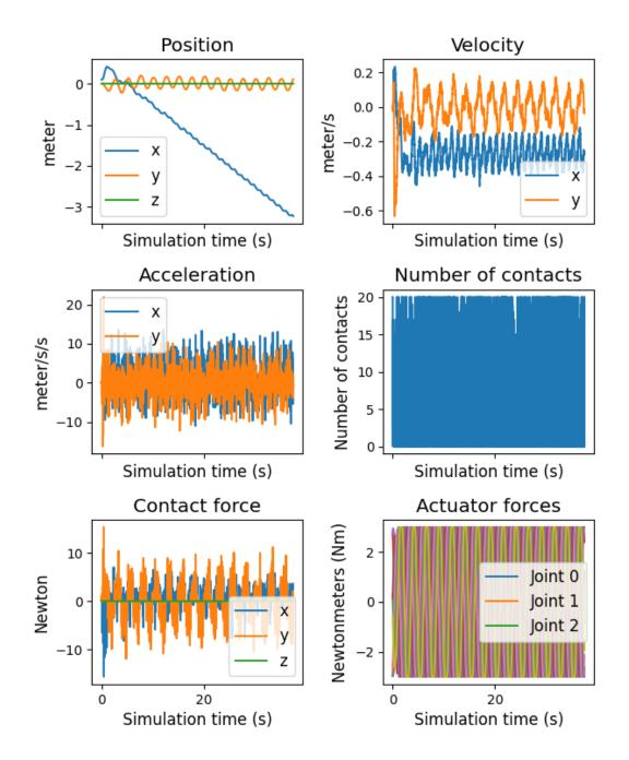
Figure 32: Lateral undulation experiment for snake robot over 40 seconds. The first row of the plot shows the head's position and velocity during the experiment. The second row shows the head's acceleration and the total number of contacts present in the simulator at any given time. The third row shows the measured contact forces for the head during the experiment as well as the actuator forces for each actuator.
