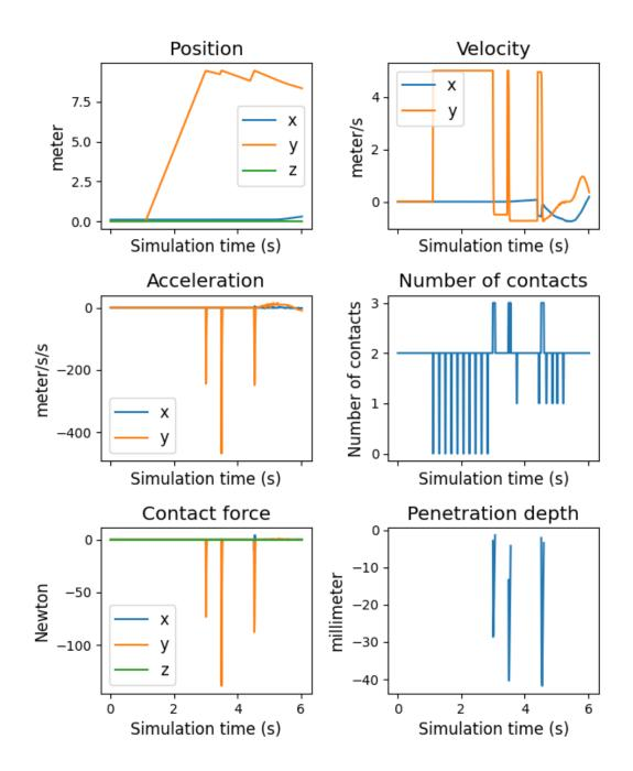
Figure 27: Collision test for one linkage with a collision along the y-axis. The first row of the plot shows the head's position and velocity during the experiment. The second row shows the head's acceleration and the total number of contacts present in the simulator at any given time. The third row shows the measured contact forces for the head during the experiment and how far the head penetrated the cylinder during the collision.
