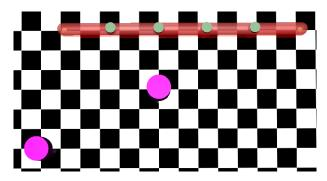
Figure 23: Configuration two showcasing a 5-linked snake. The gray objects along the snake are actuators that have been set to be visible to showcase the joints
