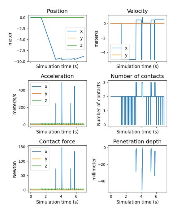
Figure 26: Collision test for one linkage with a collision along the x-axis. The first row of the plot shows the head's position and velocity during the experiment. The second row shows the head's acceleration and the total number of contacts present in the simulator at any given time. The third row shows the measured contact forces for the head during the experiment and how far the head penetrated the cylinder during the collision.
