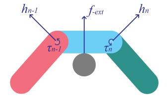
Figure 1: Forces and torques applied on a 2-jointed 2D-snake pushing up against an object. Courtesy of [6].
