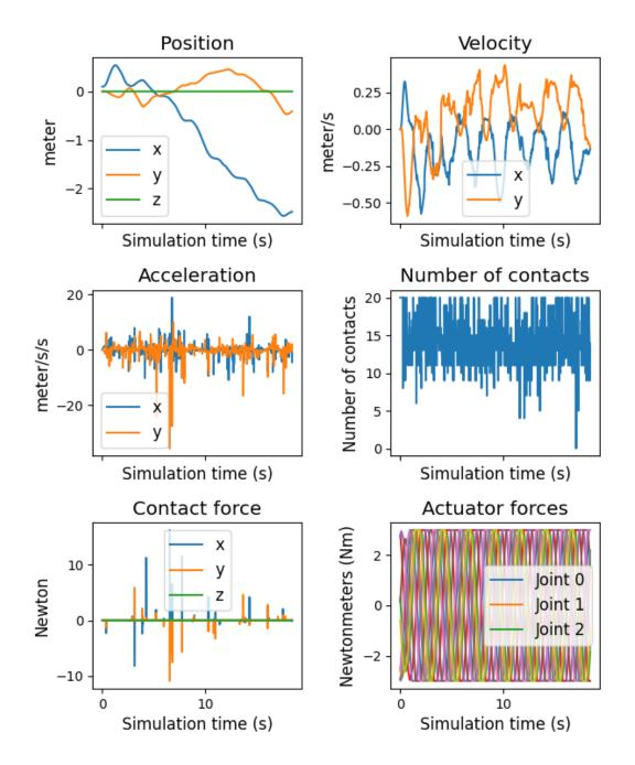
Figure 33: Lateral undulation experiment for snake robot over 20 seconds without friction. The first row of the plot shows the head's position and velocity during the experiment. The second row shows the head's acceleration and the total number of contacts present in the simulator at any given time. The third row shows the measured contact forces for the head during the experiment as well as the actuator forces for each actuator.
