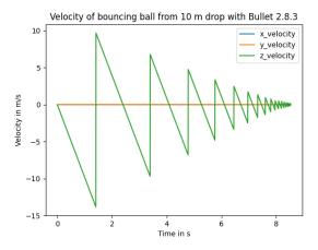
(b) Velocity graph for bouncing ball with Bullet
