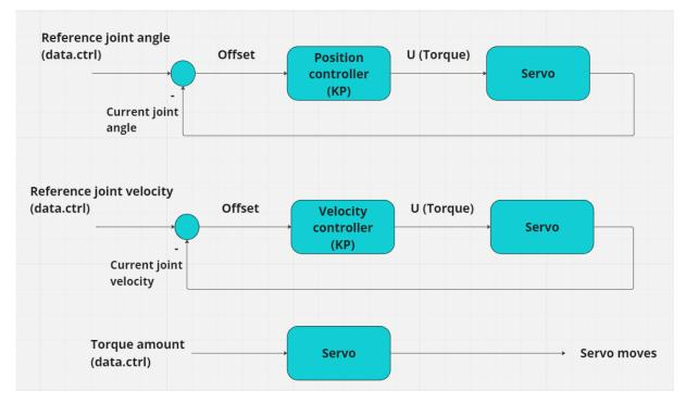
Figure 16: Diagram showcasing torque, position, and velocity control
