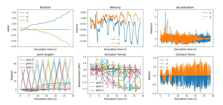
Figure 35: Form closure experiment for snake robot consisting of 16 linkages. The first row showcases the head's position, velocity, and acceleration throughout the simulation. The second row showcases the joint angles for each joint, the actuator forces for each actuator, and the contact force for the head during the simulation
