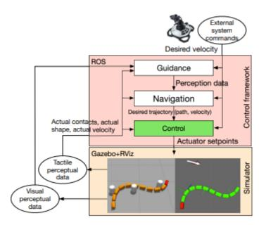
Figure 6: Snakesim software architecture, courtesy of [8]
