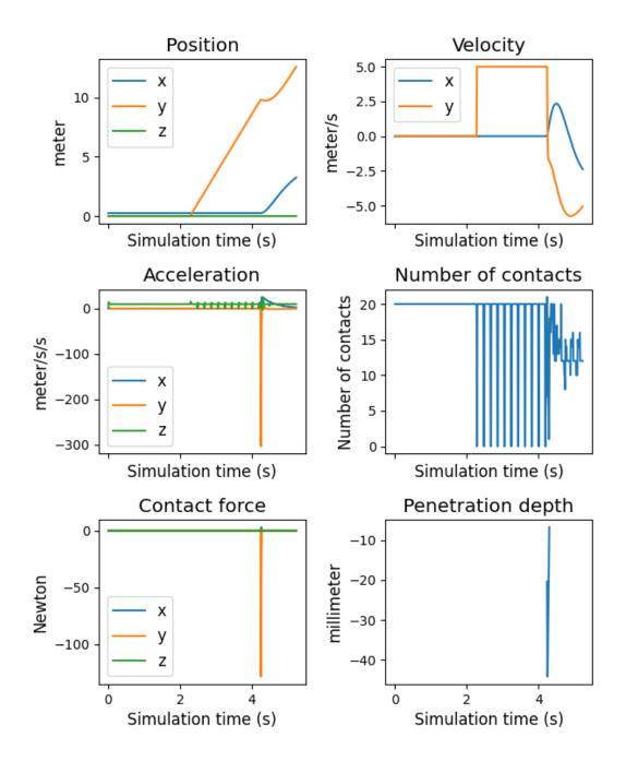
Figure 29: Collision test for ten linkages with a collision along the y-axis. The first row of the plot shows the head's position and velocity during the experiment. The second row shows the head's acceleration and the total number of contacts present in the simulator at any given time. The third row shows the measured contact forces for the head during the experiment and how far the head penetrated the cylinder during the collision.
