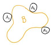
Figure 21: Figure showcasing form closure concept where object B has been completely immobilized in rotation and translation. Courtesy of [38]
