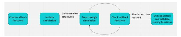
Figure 15: Main simulation loop for one run of the simulate\_snake.py python file
