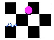
(b) Snake placement at the ending of lateral undulation experiment. The white dots on the snake are the actuators changing color based on how much torque is being used from 0 -  $\pm 3Nm$
