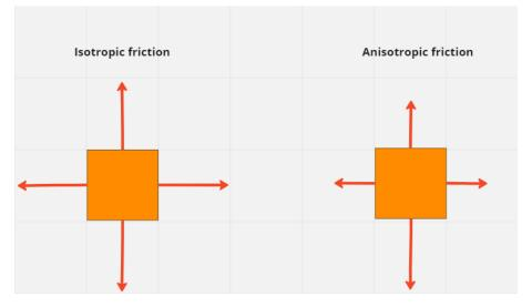
Figure 10: Example of isotropic (left box) and anisotropic friction (right box). The boxes indicate the same object, and the arrows indicate the amount of friction forces the box receives moving in each direction. One can clearly see here that when isotropic friction is present, the friction amount is the same in every direction, while this is not the case for anisotropic friction
