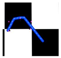
Figure 36: Snake robot performing the form closure experiment, with first-order form closure instead of second-order. The white dots are the actuators set to visible to showcase the position of the joints
