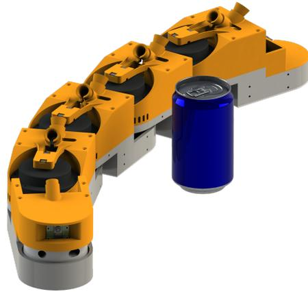
Figure 4: The Boa snake robot, courtesy of [5]
