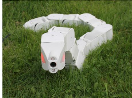
Figure 2: The Mamba snake robot, courtesy of [7]
