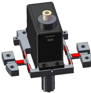
(a) 3D-model of an older version(v0) of the force-torque measurement system
