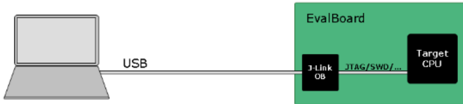
Figure 2.5: Connecting a computer and the target CPU using a Jlink OB[2]
