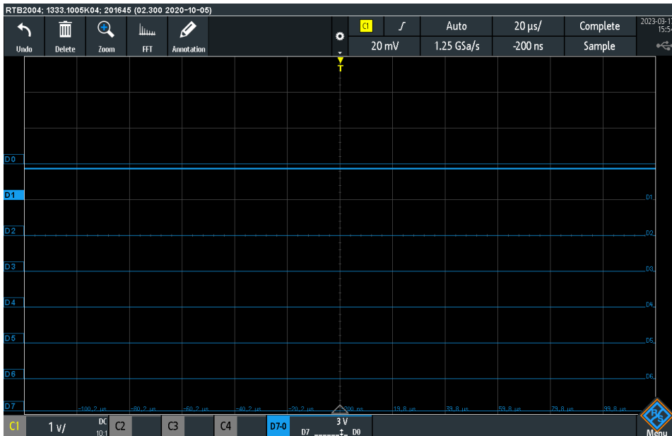
Figure 4.11: Capturing attempt to set SPI pins in high state
