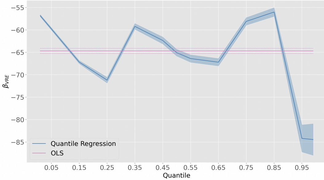
Figure 23: Gradients for VRE across price quantiles in a system with varying levels of both BSS storage and VRE capacity.
