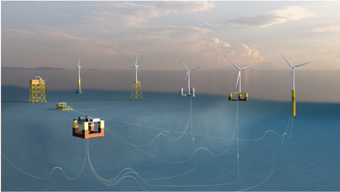
Figure 2.3: A CS for an OWPP, with both bottom-fixed and floating WTs connected to OSSs via underwater cables. The OSSs are either floating or bottom-fixed, depending on the water depth [11].
