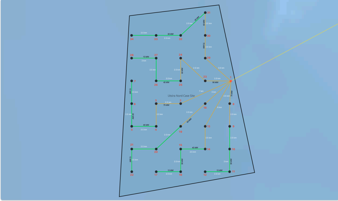
Figure 6.1: Case site CS overview with distances and power flows given no losses, produced using Vind [49].
