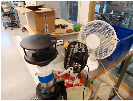
Figure 23: The fans setup to simulate true wind and head wind as the velocity of the boat was changed.
