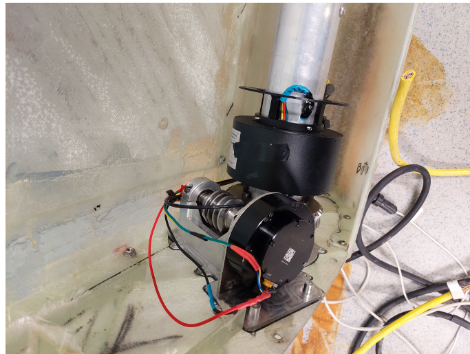
Figure 12: Inside the sail: the actuator and the position sensor.
