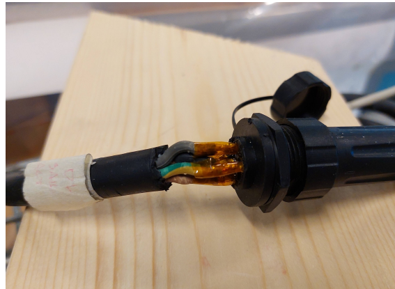
Figure 28: Example of good solder with enough heat and covered with an isolating, heat resistant material.
