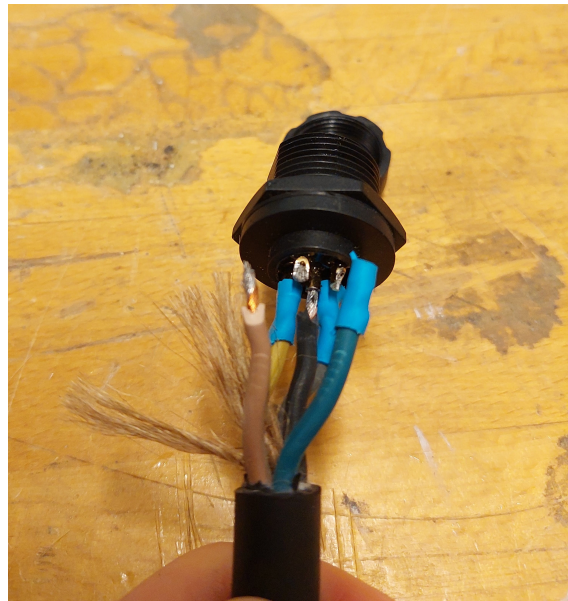
Figure 27: Example of brittle solders breaking.
