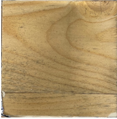
Figure 5.29 Sample 7-3 showing a spline in the surface.
