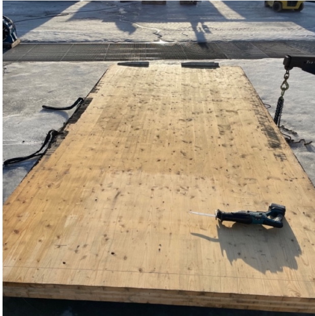
Figure 2.9 The back of a ceiling element from the compartment test. The unexposed back is used to cut samples used in the cone calorimeter tests.
