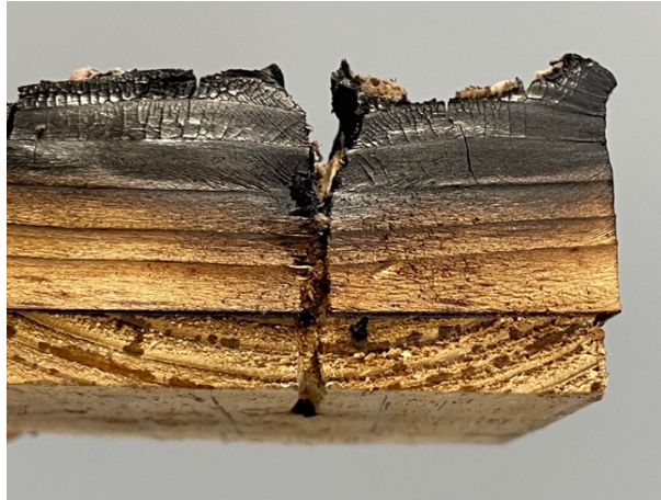
Figure 6.2 Showing cracks at the same place a TC in Test 1-2.
