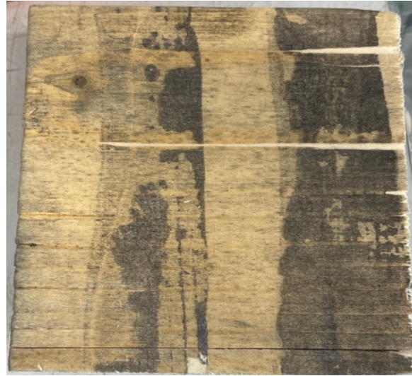
Figure 6.6 Irregularities and a spline in the surface in Test 7-4.
