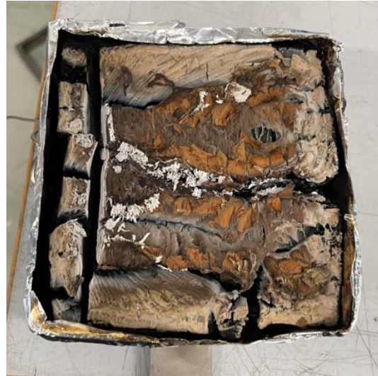
Figure 5.6 Test 2-2 showing cracks of char on the same side as the burning continued.
