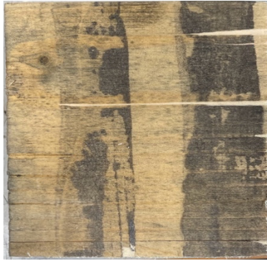
Figure 5.30 Sample 7-4 showing irregularities in the surface.
