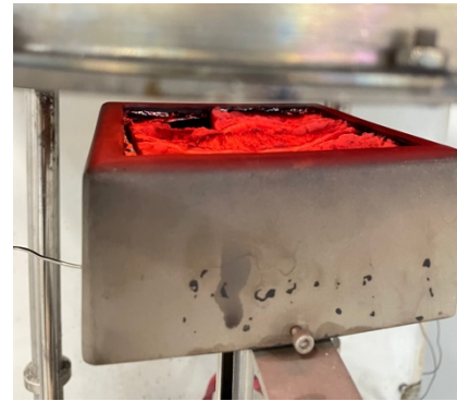
Figure 5.15 Sample 4-2 during the test with no ignition in Phase 1 and 1.2.
