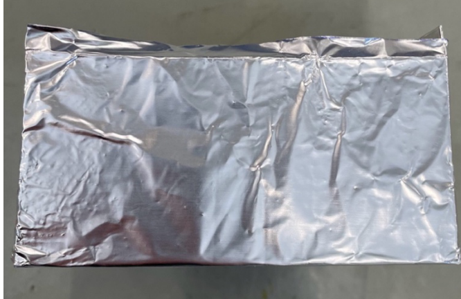
Figure 2.10 CLT sample inside the aluminum foil before testing seen from the side.
