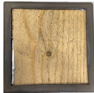
Figure 5.23 Surface of sample 5-3 showing a twig in the middle of the sample.
