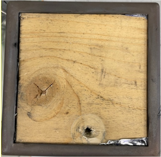
Figure 6.5 Holes and twigs in the surface in sample 4-3.
