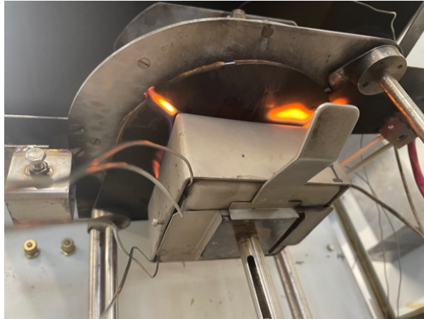
Figure 5.3 Observations from Test 1-3, when the flames went around the lid in Phase 2.
