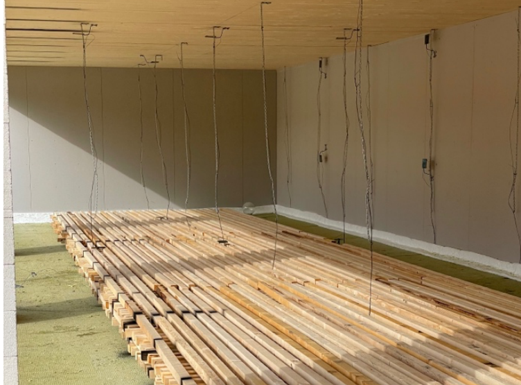
Figure 2.2 Wood crib inside the compartment representing a fuel load for an office or living room area.
