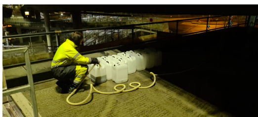
Figure 8: Collection of wash water at the Vålerenga tunnel
