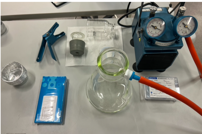
Figure 10: Filtration setup used for precipitation and TSS.
