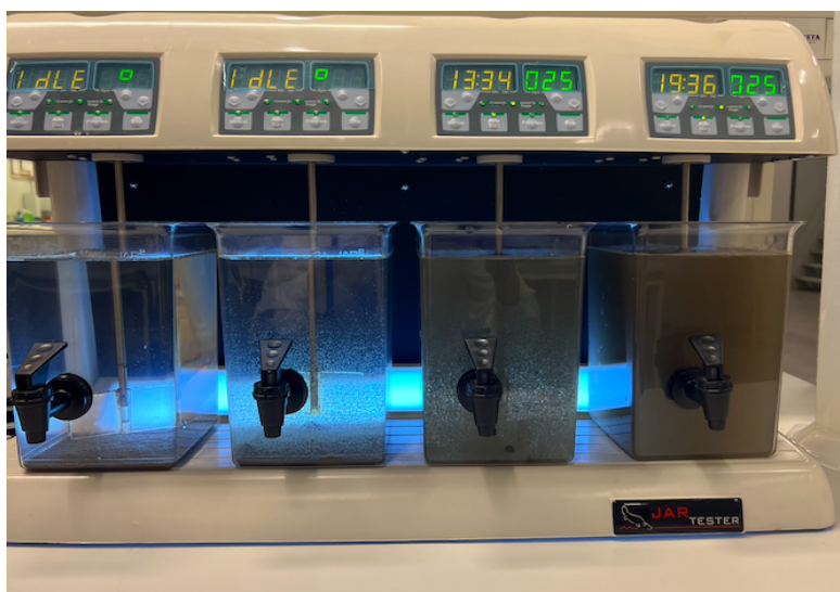
Figure 12: Setup of the jartest used for coagulation and precipitation.
