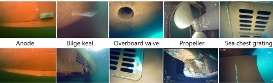
Fig. 3. Visualization of the class labels of LIACI
