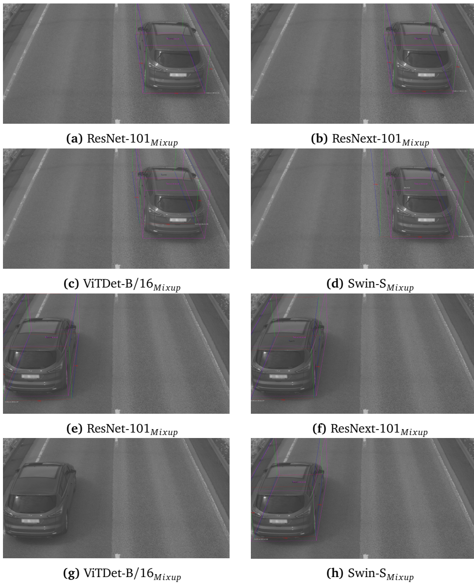
Figure 4.4: Predictions and ground truth (purple bounding box) for the four models utilizing the standard Mixup approach on the rear view.
