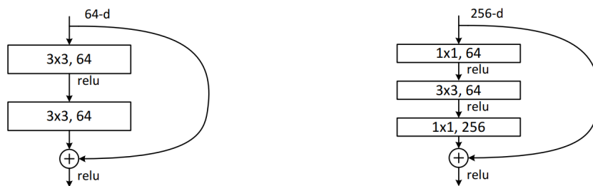
(a) Basic building block consisting of two convolutional layers. Used in ResNet-18/34
