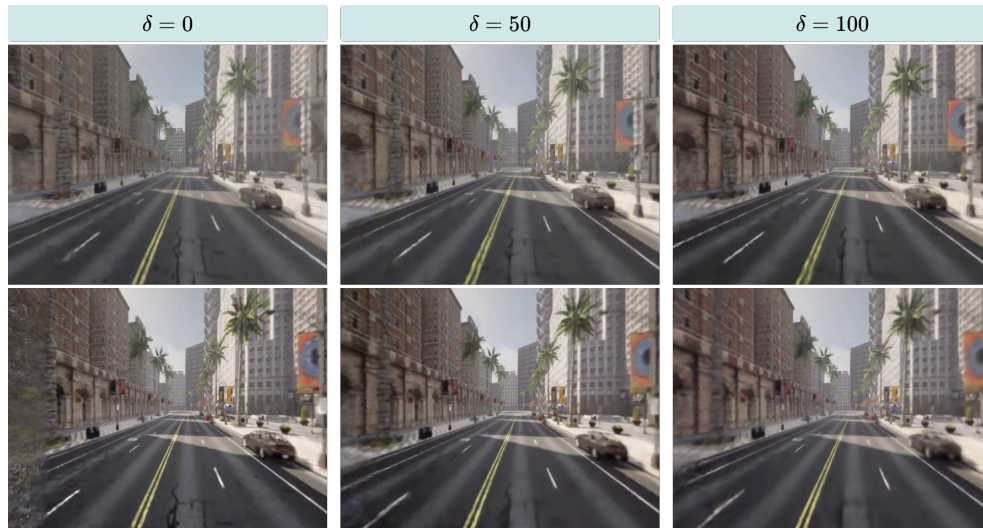
Figure 4.7: Comparison of Block-NeRF trained with 0, 50 and 100 images overlap, respectively. The top row corresponds to the last frame rendered by Block-NeRF number 0. The bottom row is the first frame rendered by Block-NeRF number 1.
