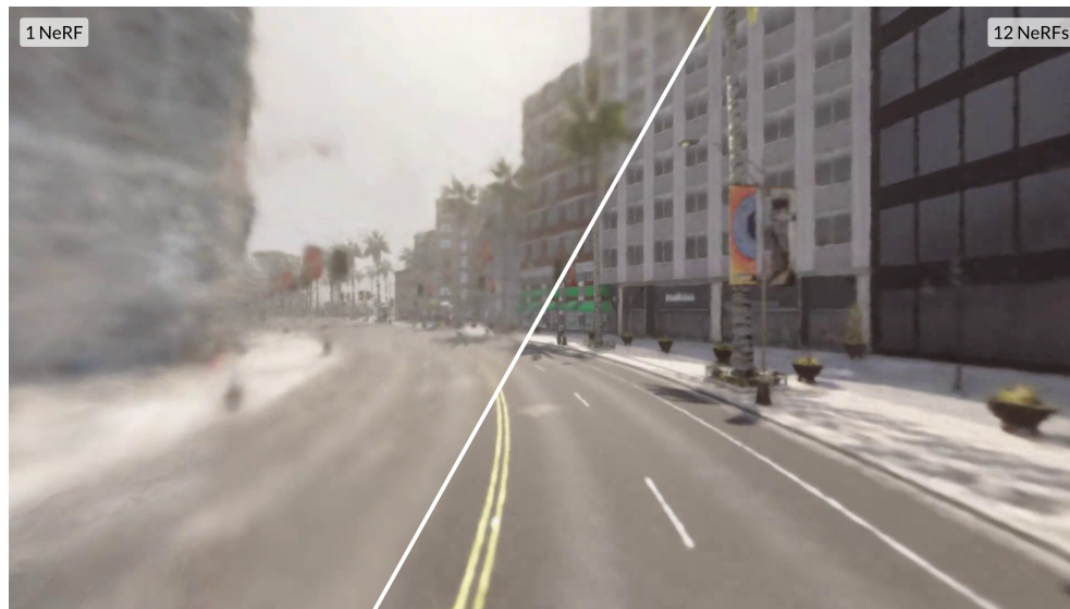
Figure 4.5: Comparison of two renders from models that have been trained on the same dataset. Left) A single NeRF trained on the full dataset, Right) 12 Block-NeRFs trained on equally spaced segments of the dataset.
