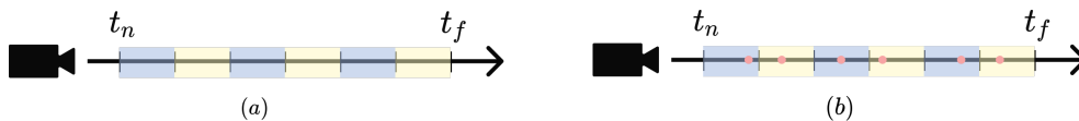
Figure 2.3: Illustration of stratified sampling. a) The ray is uniformly binned from the near bound t_n to the far bound t_f of a ray \mathbf{r}(t) , defining the strata. b) A single random point is randomly sampled from each stratum.
