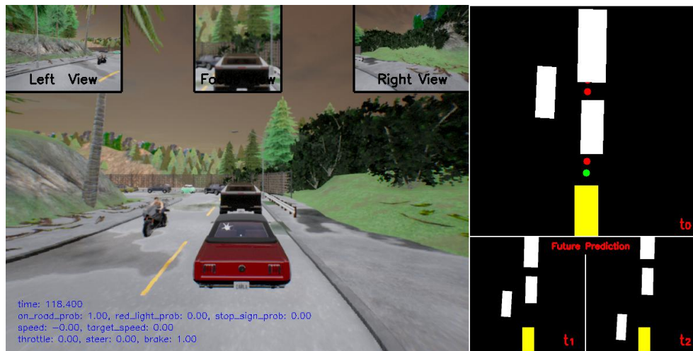
Figure 4.3: Visualization of model inputs and outputs for IF-pretrained evaluated on the first route of Longest6 in CARLA 0.9.10. Left: The camera inputs. The largest image shows the center view. In the top left and top right we have the left and right views. The top center image is the focus view, which is a middle crop of the large center view. Right: The agent’s predicted object density map, consisting of predicted vehicle and pedestrian bounding boxes for the current and two future time steps, as well as predicted waypoints for the current time step. The waypoints are green if the path is predicted to be clear, and red if the model thinks there are objects in the way. Bottom left text: The agent’s predicted traffic rule information including whether the car is on the road, if it predicts a red light, and if it predicts a stop sign ahead. It also shows the current throttle, steering, and braking commands, as well as the current and target speed. A video of this evaluation is available at https://youtu.be/TK3uwBmQh54?t=26&list=PLWGD02Z_62kKDze_p2hgt8DFM0e3VElga .
