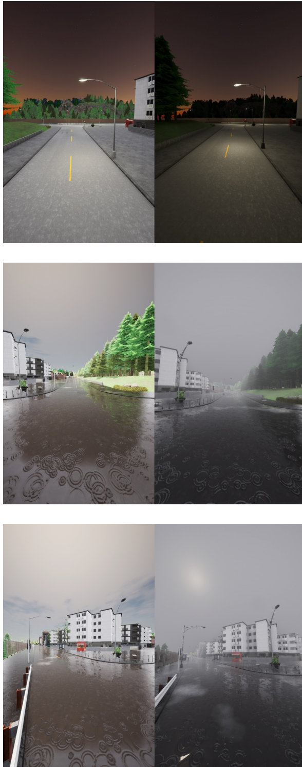
Figure 3.16: Three examples comparing the graphical differences between CARLA versions 0.9.10 (left) and 0.9.14 (right). In general, there is less ambient light and the fog is more dense. Additionally, CARLA 0.9.14 features a new effect where rain drops on the camera lens can distort parts of the image (lower right).
