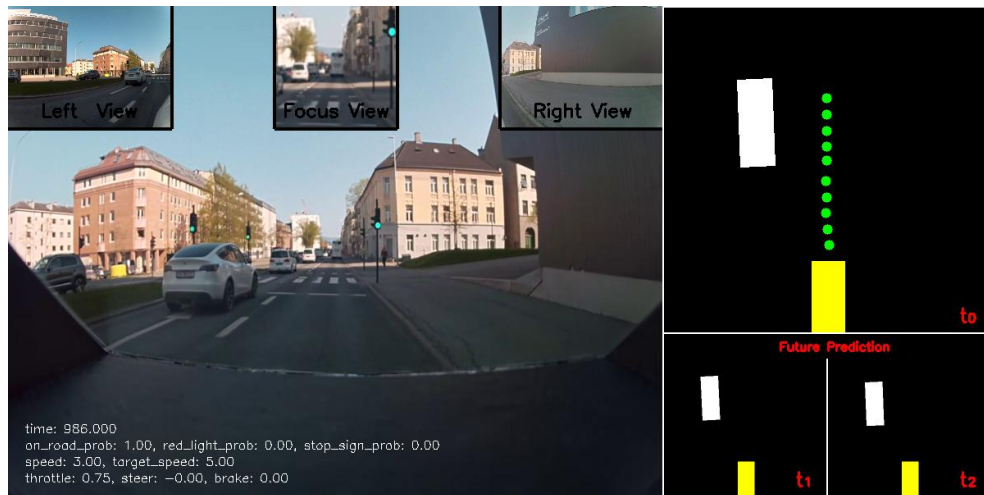
(b) IF-ds-kia. Here we see the different mechanism of camera input, as different sensors instead of stitched together into one. The model accurately predicts the bounding box for the closest car, as well as correct predictions for 1) being on the road, 2) seeing a red light, and 3) seeing a stop sign.
