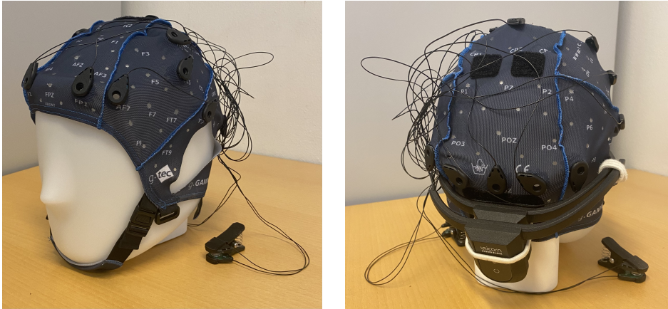
(a) The Unicorn Hybrid Black electrodes with the g.GAMMAcap from g.tec.
