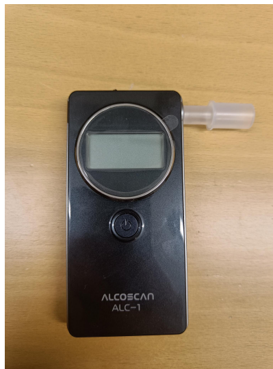
Figure 3.7: Alcoscan ALC-1, the breathalyser used to measure the BAC of the participants [1].
