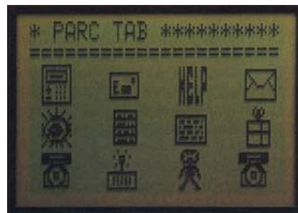
Figure 13: GUI displayed on a portable device, developed by Xerox Palo Alto Research Center, which may be connected to a variety of workstations.
