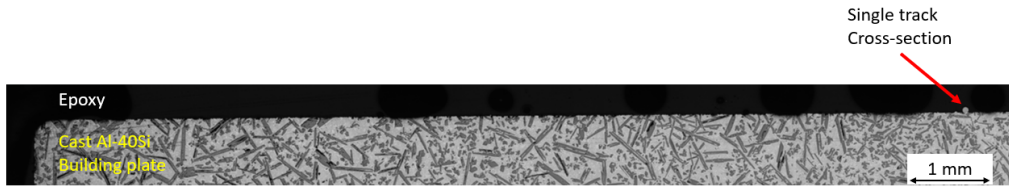
Figure 50: Example of an OM panorama image of the Al-40Si building plate cross-section conducted with the Zen Core software.
