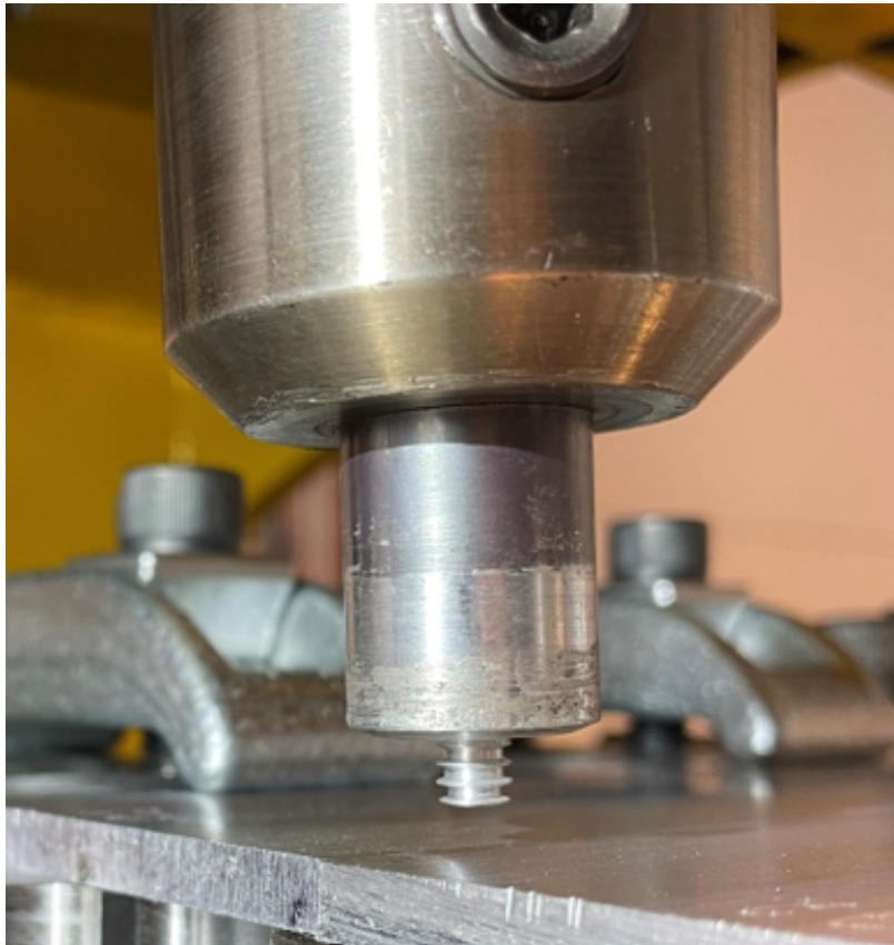
Figure 22: A picture of the welding tool used in the friction stir welding experiments.
