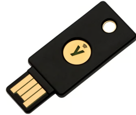
Figure 2.2: A security key, more specifically a YubiKey. It is USB-compatible and has a touch sensor in gold on top.
