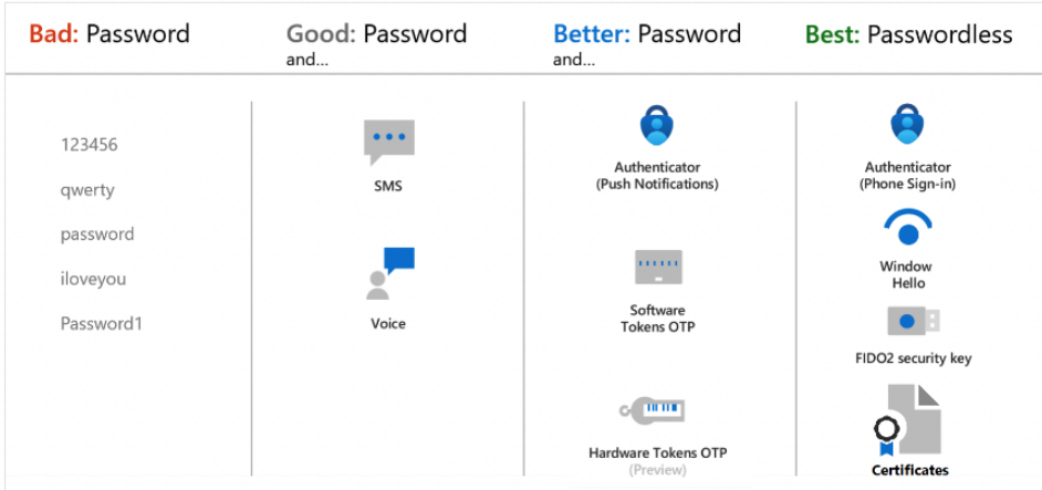
Figure 2.4: Ranked authentication methods by [Mic23]. Passwords are bad, passwords in combination with other factors are better, and passwordless is the best.
