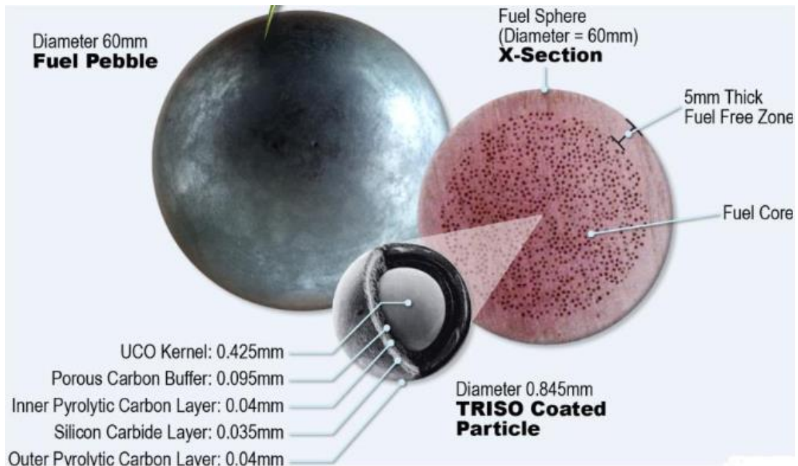
Figure 11 Characteristics and composition of the TRISO fuel pebbles manufactured by X-energy[52].
