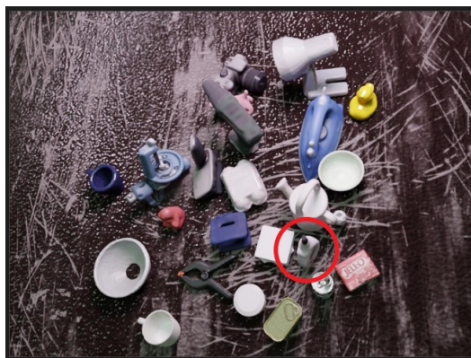
Figure 7.3: An example of what a synthetic image from the LMO dataset looks like. The image has dimensions 640x480. A red circle is added to highlight the glue, and is not a part of the original image. The glue is displayed by 1050 pixels and has a visible fraction of 100%. Most methods use a separate object detector to zoom in on the object of interest during inference. In this image the gorilla figurine(red), the cat object(pink behind the screwdriver) and the stapler object(blue) are shown. These will be used for testing.
