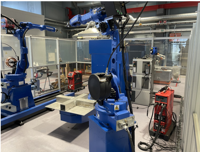
Figure 3.8.: The image captures the complete robot cell, which includes two robot arms, a linear module (TSL600), a workpiece positioner module (MT1), and two welding apparatus.
