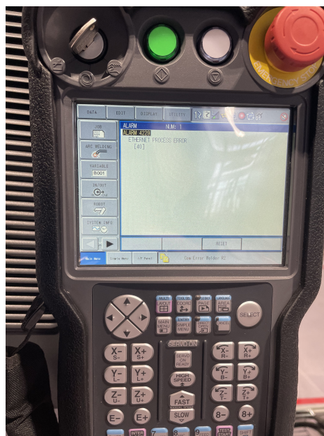
Figure 8.7.: If no Ethernet connection is detected after MotoROS2 is installed on the controller, a warning will show.
