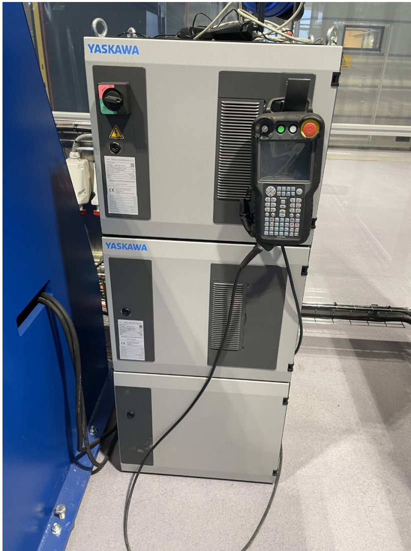
Figure 3.1.: The Motoman YRC1000 robot controller with the teach pendant (top right corner of the controller).
