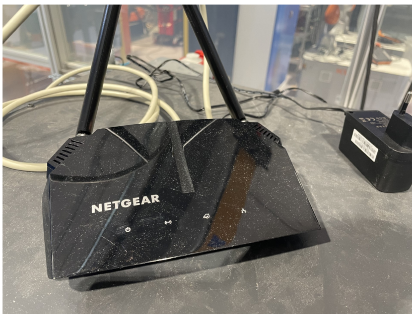
Figure 3.2.: Netgear R2610 wireless router used for establishing network connectivity in the setup.
