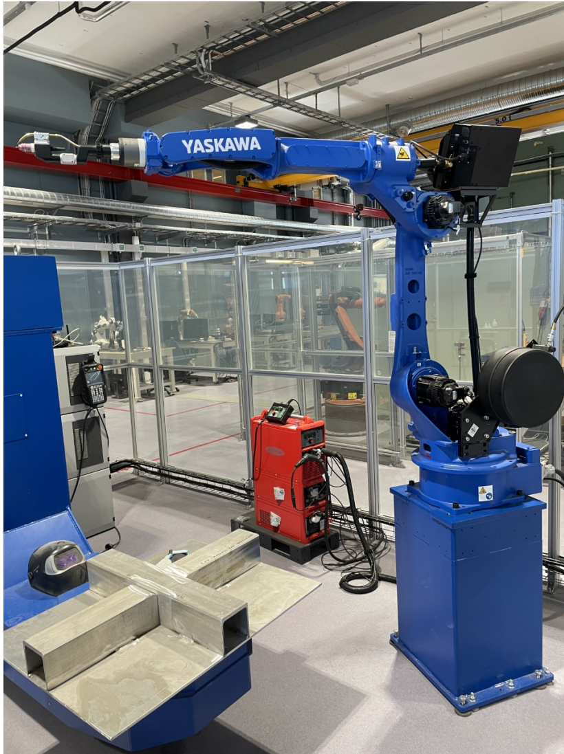
Figure 3.3.: Yaskawa Motoman GP 25-12 industrial robot arm equipped with TIG torch as end effector.
