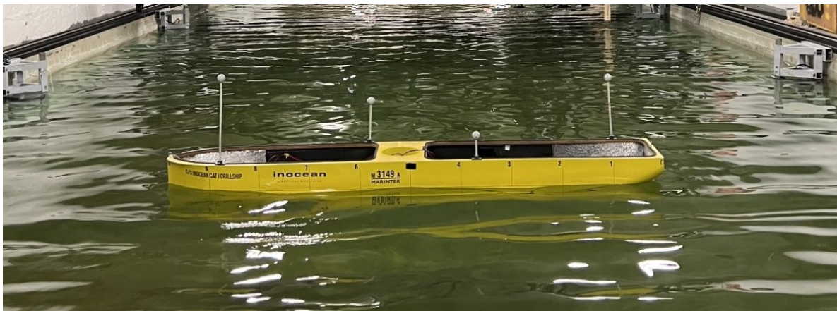
Figure 2.17: CSAD in the wave basin in the MC-lab.
