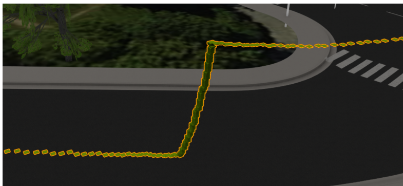
(d) Errors in altitude readings occurring while the vehicle stands still.
