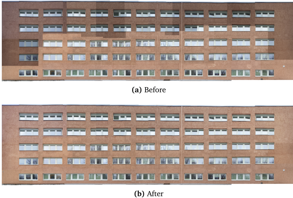
Figure 13.2: Before and after performing exposure and saturation correction on a stitched image textures.
