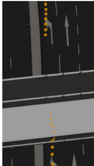
(c) Missing GNSS readings caused by obstacles between the vehicle and GNSS satellites.
