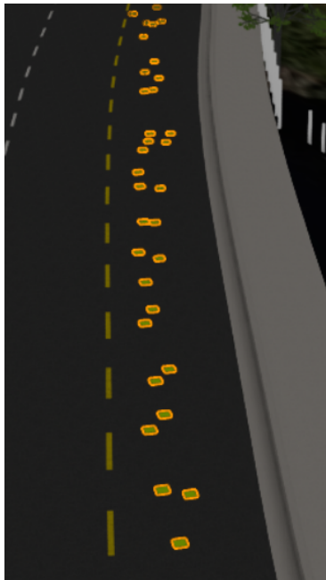
(b) Jitter in the GNSS readings caused by obstacles between the vehicle and GNSS satellites.
