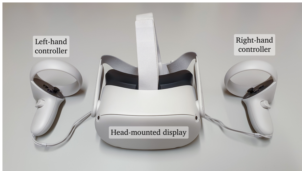
Figure 2.10: Illustration of the most important hardware components of a VR suite. The suite shown is called Meta Quest 2.
