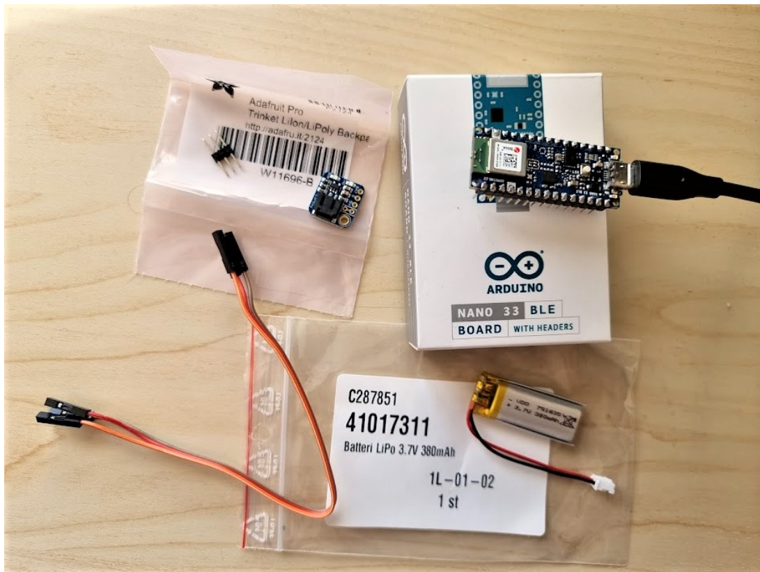
Figure 5.25: Parts used for making Arduino wireless: LiPoly Backpack, simple cables for testing, Arduino itself and battery LiPo.
