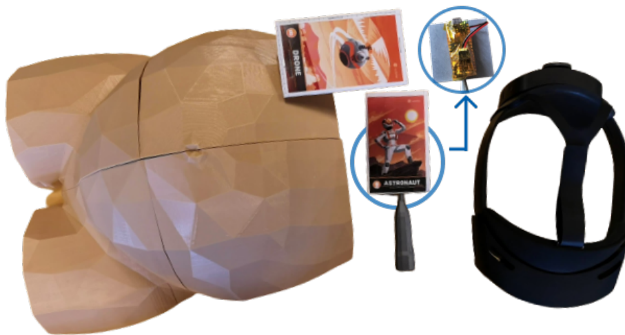
Figure 6.1: The components needed for HoloUmoja application: 3D printed abdomen and probe (the sensor is behind the tracking images) with Vuforia Image Targets and HoloLens 2
