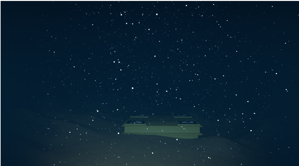
Figure 4.10: A render of snow particles added to VAROS in blender. A particle system emitting spheres of fixed size was used (essentially the most basic implementation).
