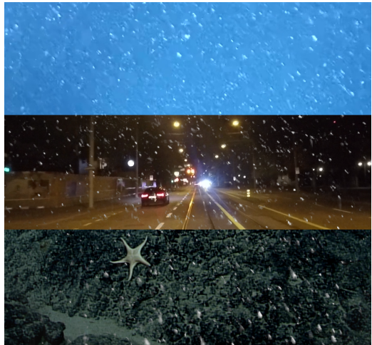
Figure 1. In our approach, we extract marine snow from underwater footage with untextured background (top), and superimpose this snow on arbitrary footage to create labelled training data (bottom images) for training snowflake detectors .
