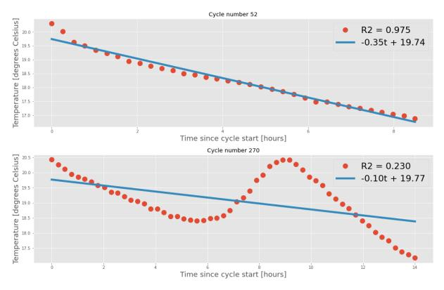
**Figure 5.2:** Typical temperature drop during OFF-cycles for winter (top) and spring (bottom). Taken from the Python script's plotting.
