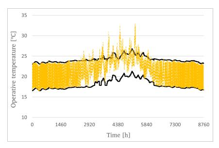
**Figure 3.12:** Operative temperature of a whole-year simulations, with the adaptive thermal limits that decided when the heater was turned on/off.
