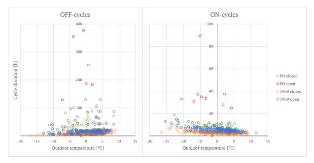
**Figure 4.6:** Cycle duration as a function of outdoor temperature for the 1969 envelope, with PH as a comparison. The cycle duration is capped at 400 hours.
