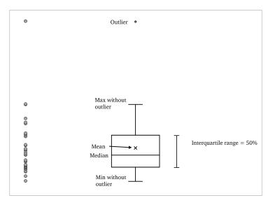
Figure 2.2: A set of values (left) and its box plot (right).
