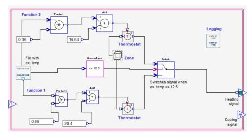
**Figure 3.13:** A custom macro for the heater received from a PhD-student at NTNU. It is based on a comfort temperature curve and uses adaptive thermal limits to determine when to turn off/on.
