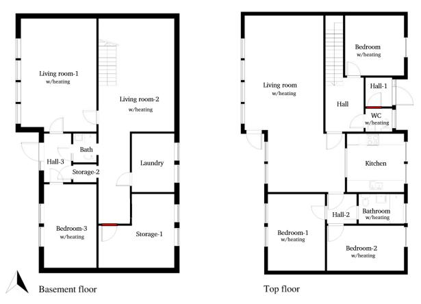
**Figure 3.10:** The floor plans of both floors, now showing which zones had heating units. The red doors are the only two doors kept closed during the second set of simulations.
