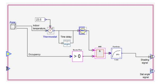
Figure 3.6: The macro for blind control, that emulates a realistic occupant behaviour (Felius, 2021).
