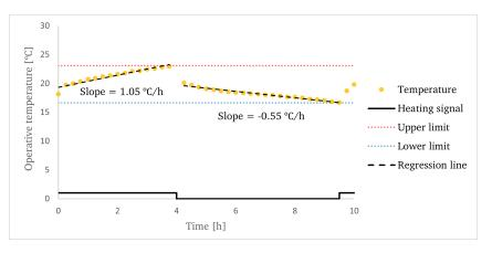
Figure 3.11: Example of two cycles, one ON-cycle and one OFF-cycle.
