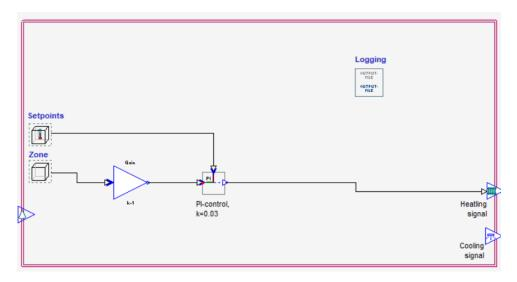
Figure 3.3: Custom macro for the heater. A replica of the built-in PI-controller.
