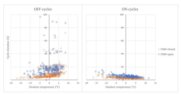
Figure 4.5: Cycle duration as a function of outdoor temperature for the 1969 envelope.
