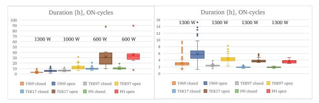
**Figure 4.4:** Duration of the ON-cycles. The left figure shows the duration with the original heating power, and the right figure shows the duration with equal heating power.
