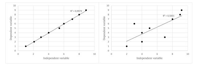
Figure 2.3: Linear regression of two different scatter plots, illustrating how the coefficient of  $R^2$  works.
