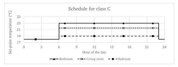
Figure 3.7: Schedule for the set-point temperature, showing the night setback for efficiency class C.
