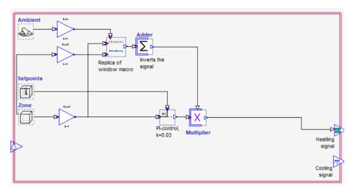
Figure 3.8: The new custom macro for the heaters, with an added window/heater interlock.
