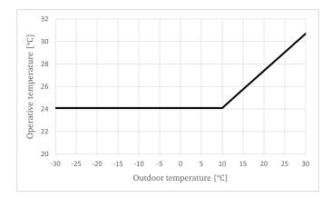
**Figure 3.5:** Set-point temperature for window opening, based on the adaptive thermal comfort model's upper limit (Norsk Standard, 2019).
