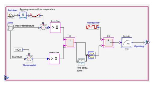
Figure 3.4: The macro for window opening, that emulates a realistic occupant behaviour (Felius, 2021).
