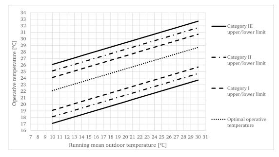
**Figure 2.1:** The adaptive comfort model from NS-EN 16798-1 (Norsk Standard, 2019). The middle line shows the preferred temperature, and the others are the upper and lower limits depending on the comfort category.
