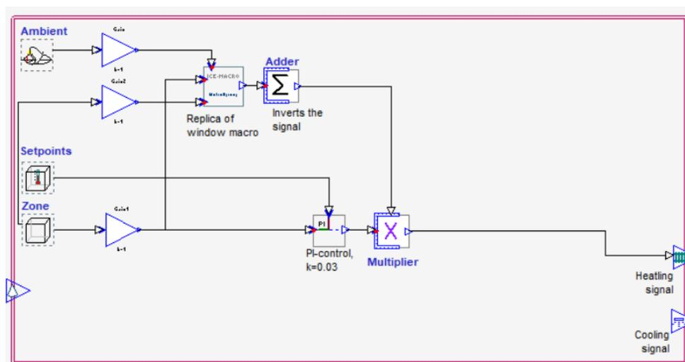
Figure 3.8: The new custom macro for the heaters, with an added window/heater interlock.
