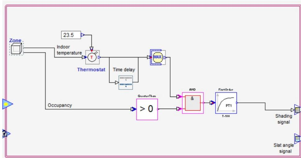
Figure 3.6: The macro for blind control, that emulates a realistic occupant behaviour (Feliu, 2021).
