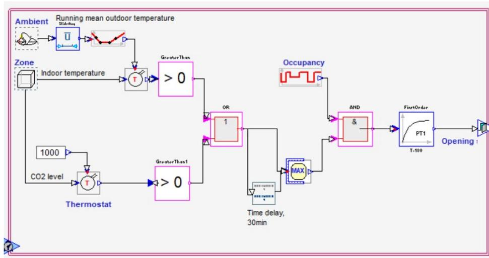
**Figure 3.4:** The macro for window opening, that emulates a realistic occupant behaviour (Felius, 2021).
