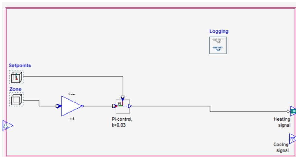
**Figure 3.3:** Custom macro for the heater. A replica of the built-in PI-controller.
