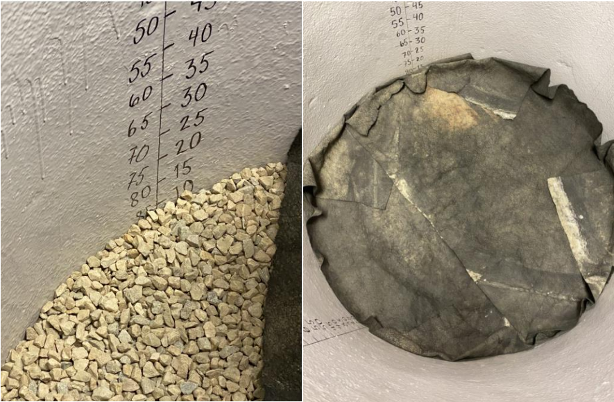
Figure 1: Base layer of gravel and filter cloth
