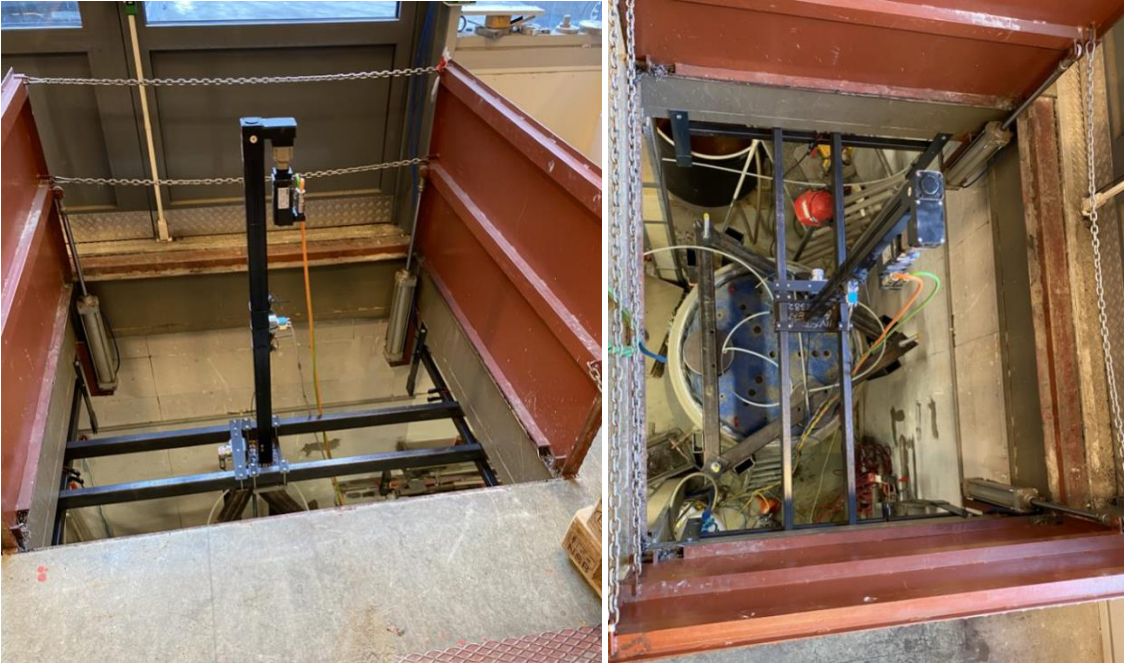
Figure 8: The setup for CPTU-testing. Showing the actuator set up.
