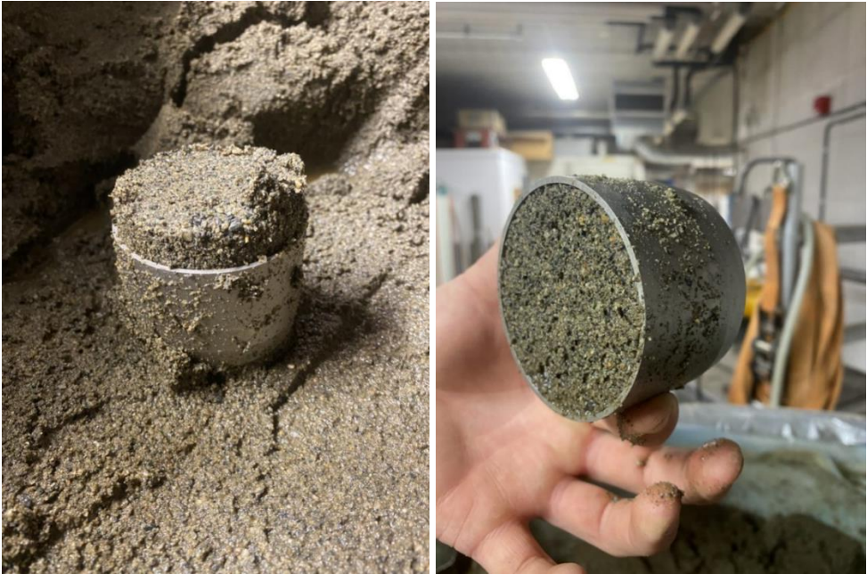
Figure 10: Density tests are sampled for each layer of 10 cm.
