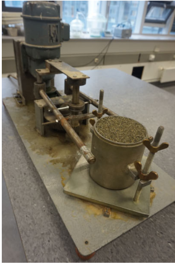
Figure 3.12: The equipment used for determining the void ratio limit, e_{min} according to the procedures suggested by DEGEBO.
