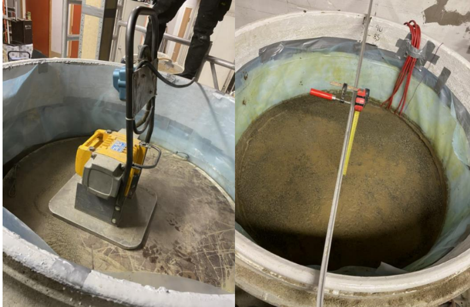
Figure 5: The sample is compacted using a plate vibrator. The final height of the layer is then measured.
