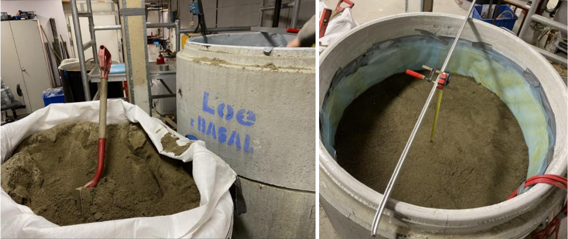
Figure 2: The sand is shoveled in at 10 cm layers each. The height of each layer is carefully measured.
