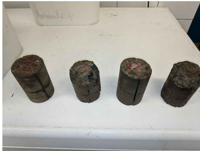
Figure A.24 Concrete samples after 2 stages of adfreeze shear tests, washed. From left to right sample #1 to #4.
