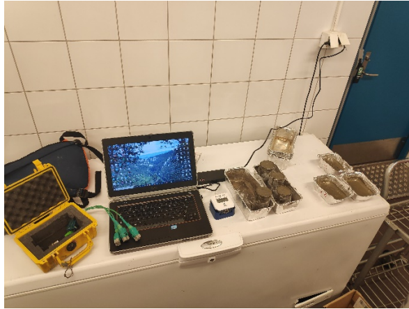
Figure A.20 Preparation of the concrete samples: middle – concrete cylinders and most right samples - thermally measured with the thermocouples.
