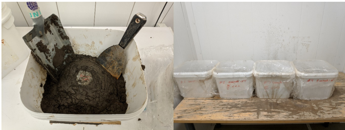
Figure A.21 Preparation of the soil samples. left (a) - sample#1 preparation and right (b) - the four soil buckets isolated and located in the cold lab
