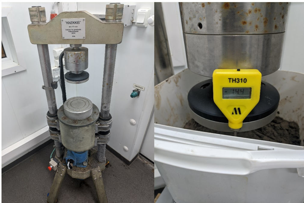
Figure A.22 left (a) - Knekkis uniaxial compression machine and right (b) - a representative figure of the setup and the measured temperature
