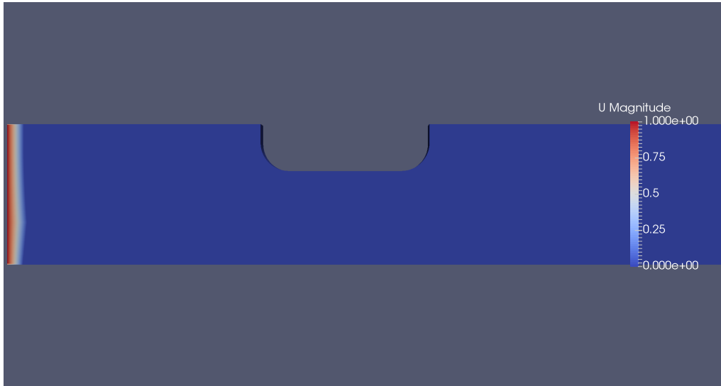
Figure B.4: Snapshot of the steady state velocity field from the simpleFoam simulation, \mathfrak{Re} = 10^5 , \frac{W_D}{T} = 3 and t = 100s
