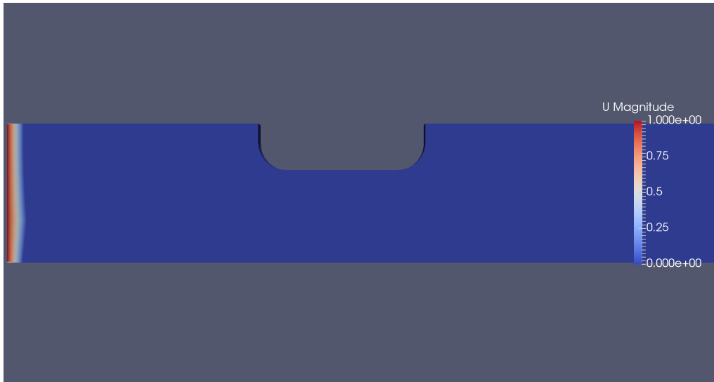
Figure B.5: Snapshot of the steady state velocity field from the simpleFoam simulation, \mathfrak{Re} = 10^7 , \frac{W_D}{T} = 3 and t = 100s
