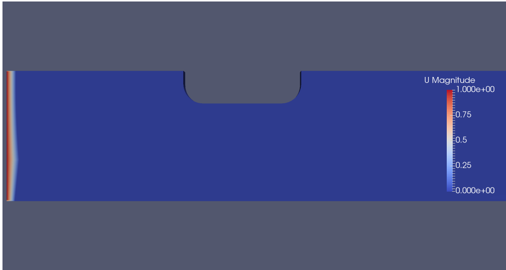
Figure B.6: Snapshot of the steady state velocity field from the simpleFoam simulation, \Re = 10^7 , \frac{W_D}{T} = 4 and t = 100s
