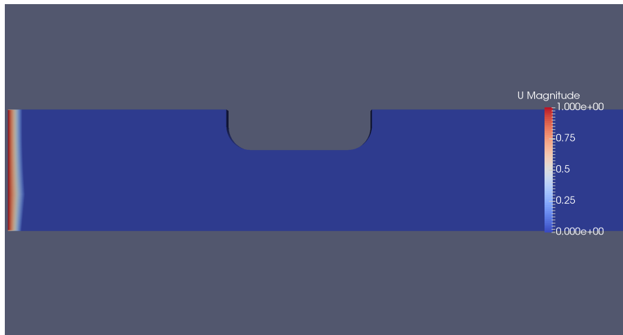
Figure 5.14: Snapshot of the steady state velocity field from the simpleFoam simulation, \mathfrak{Re} = 10^5 , \frac{W_D}{T} = 3 and t = 100s
