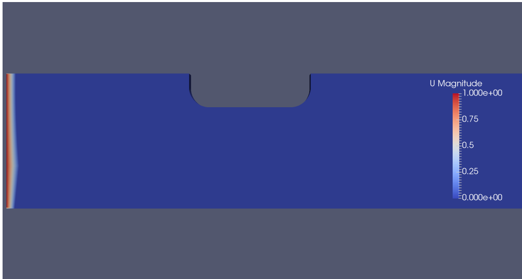
Figure B.3: Instantaneous snapshot of the velocity field from pimpleFoam transient simulation, \mathfrak{Re} = 10^5 , \frac{W_D}{T} = 4 and t = 100\text{s}
