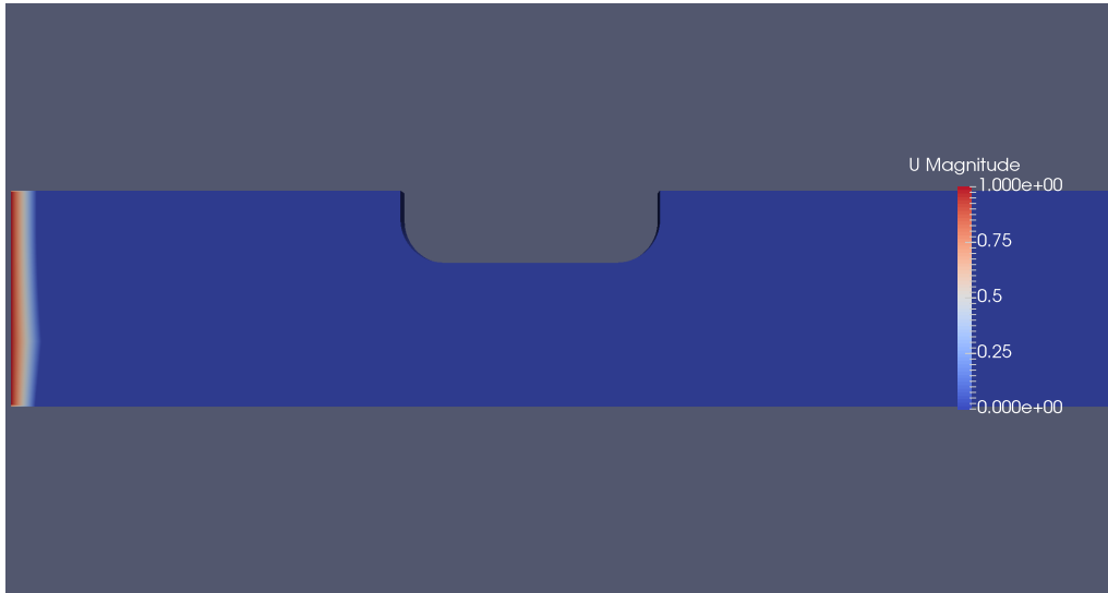
Figure B.2: Instantaneous snapshot of the velocity field from pimpleFoam transient simulation, \mathfrak{Re} = 10^5 , \frac{W_D}{T} = 3 and t = 100\text{s}
