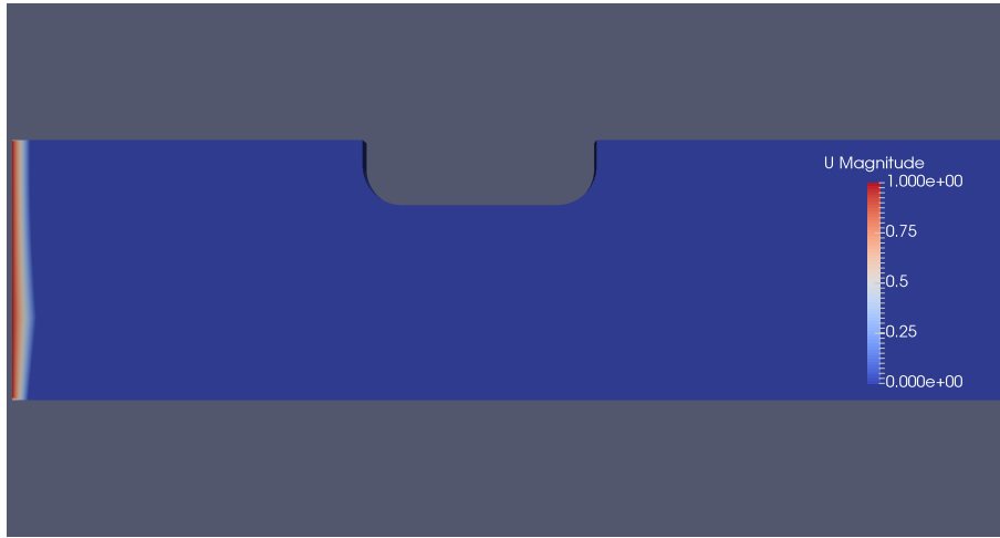
Figure 5.12: Instantaneous snapshot of the velocity field from pimpleFoam transient simulation, \Re = 10^7 , \frac{W_D}{T} = 4 and t = 100s
