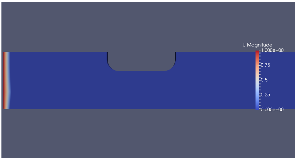
Figure B.1: Instantaneous snapshot of the velocity field from pimpleFoam transient simulation, \mathfrak{Re} = 10^7 , \frac{W_D}{T} = 3 and t = 100s
