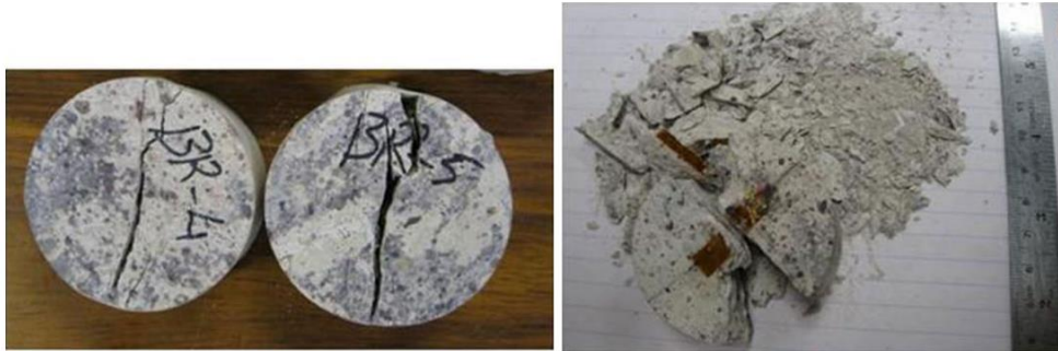
Figure 4-2: Brazilian disc specimens of Brisbane tuff after failure tested under (left) monotonic loading and (right) cyclic loading (Erarslan et al., 2014)
